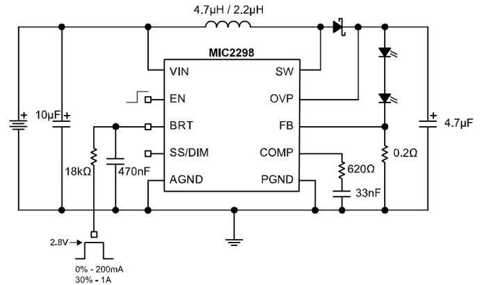
Figure 5. High Frequency PWM Programming Via BRT Pin
