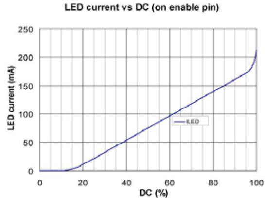
Figure 6. LED Current vs. DC (on enable pin)
