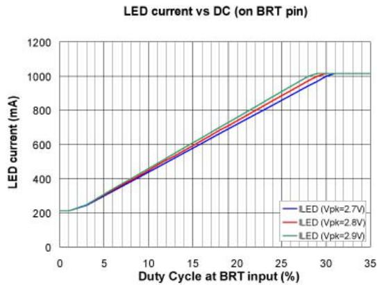
**Figure 7. LED Current vs. DC (on BRT pin)**
