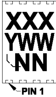
8-Lead TDFN (2 x 3 x 0.8 mm) (MCP6V37)
