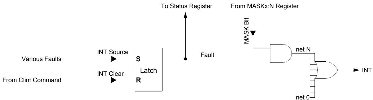
**Figure 17. Interrupt handling**
