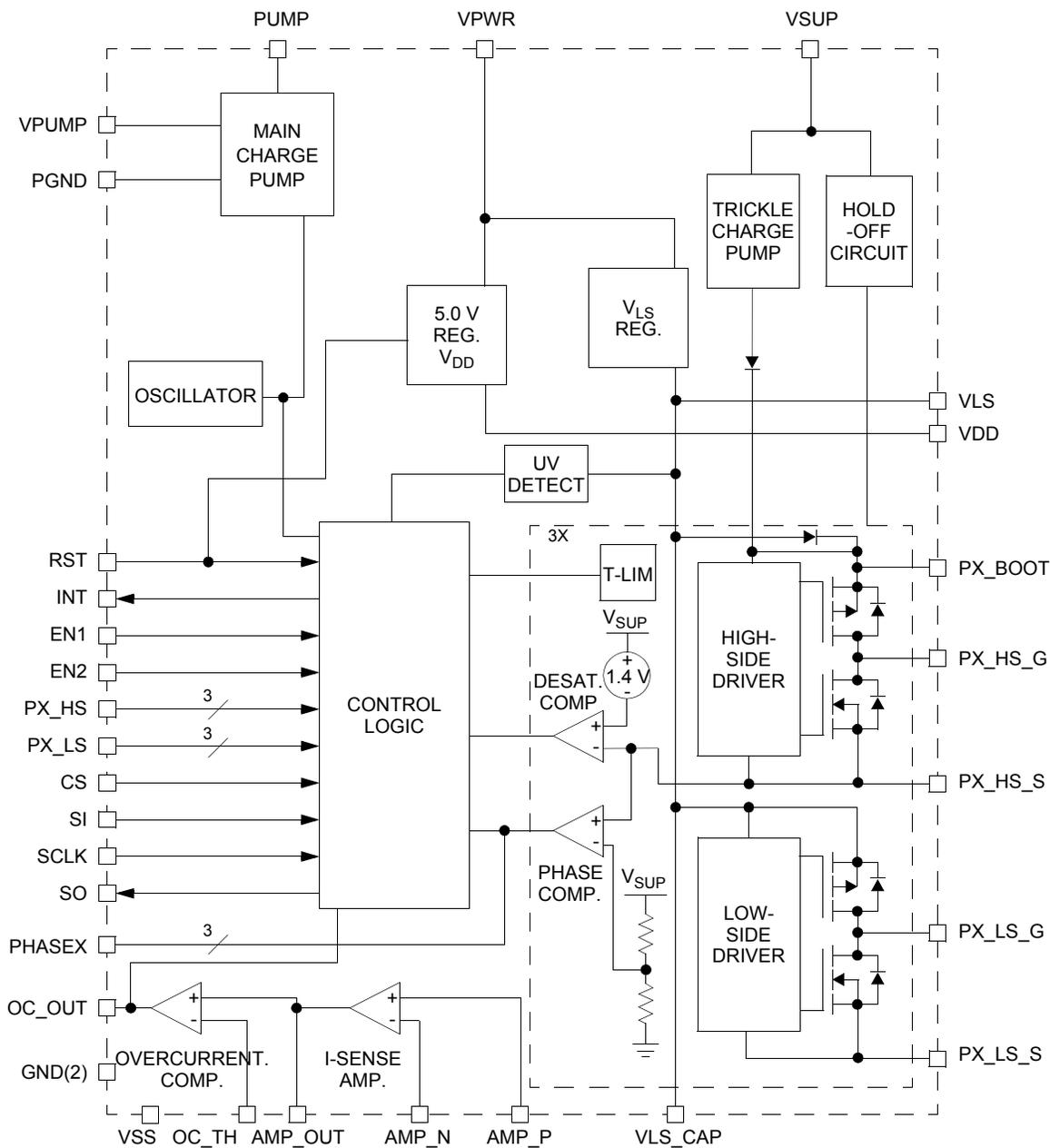
Figure 2. 34GD3000 simplified internal block diagram
