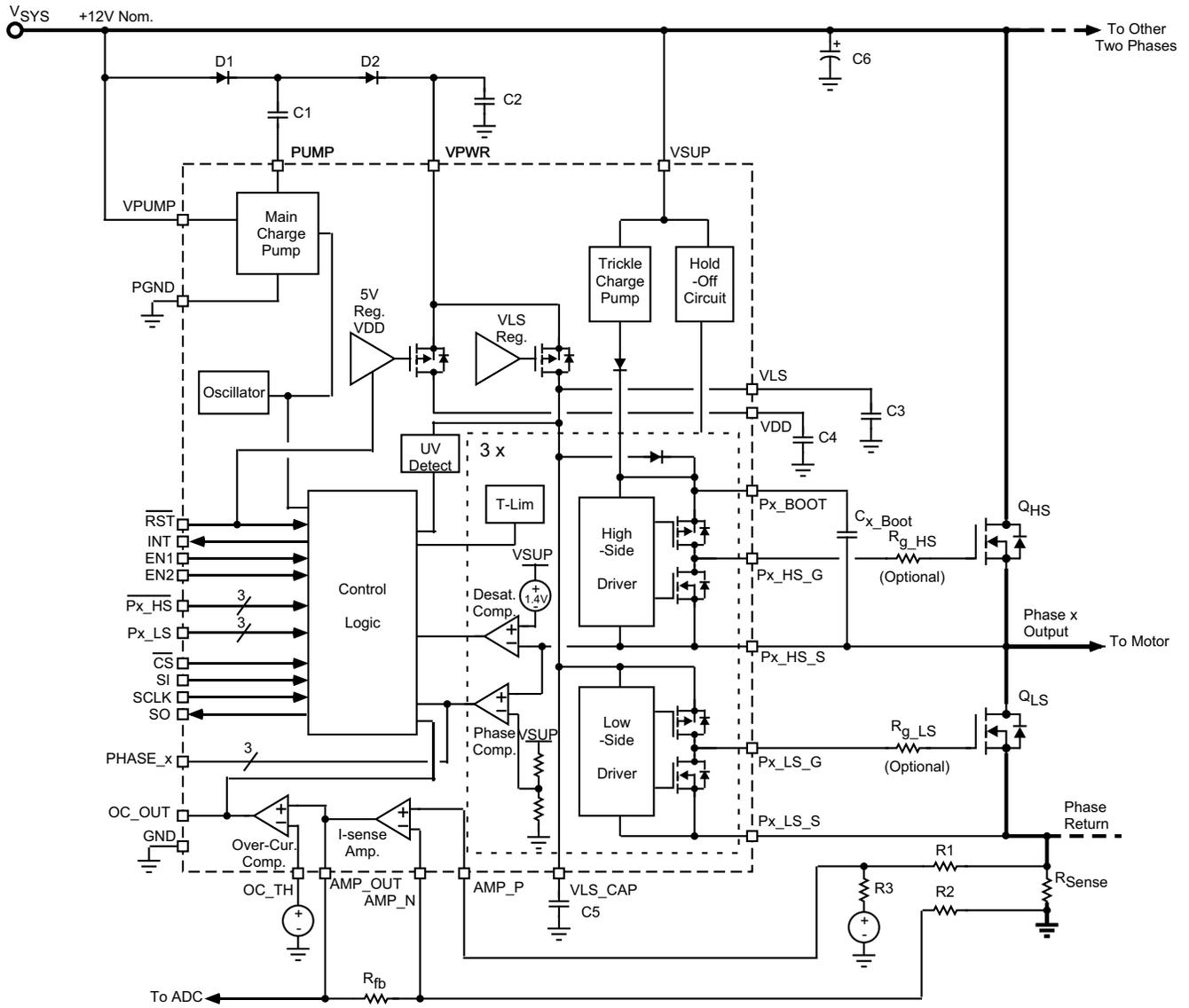
Figure 21. Typical application diagram using charge pump
