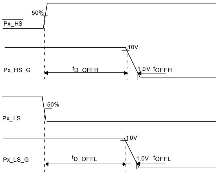
**Figure 8. Driver turn-off time and turn-off delay**
