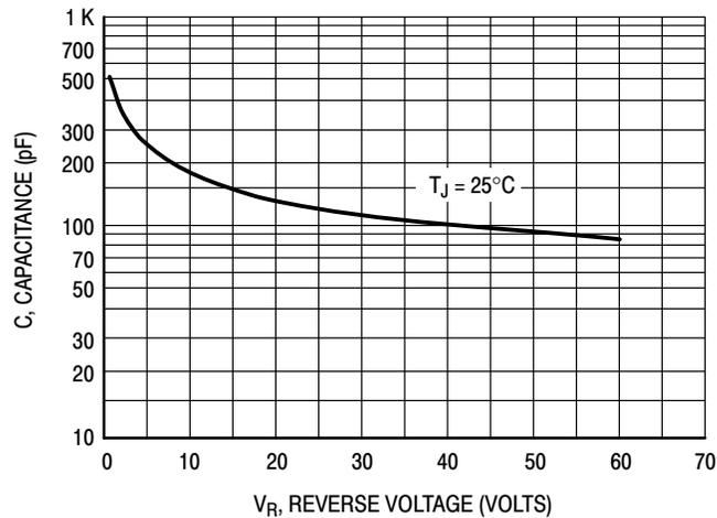
Figure 6. Typical Capacitance
