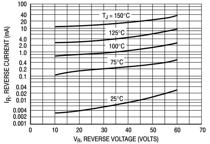
\*The curves shown are typical for the highest voltage device in the voltage grouping. Typical reverse current for lower voltage selections can be estimated from these curves if  $V_R$  is sufficient below rated  $V_R$ .
