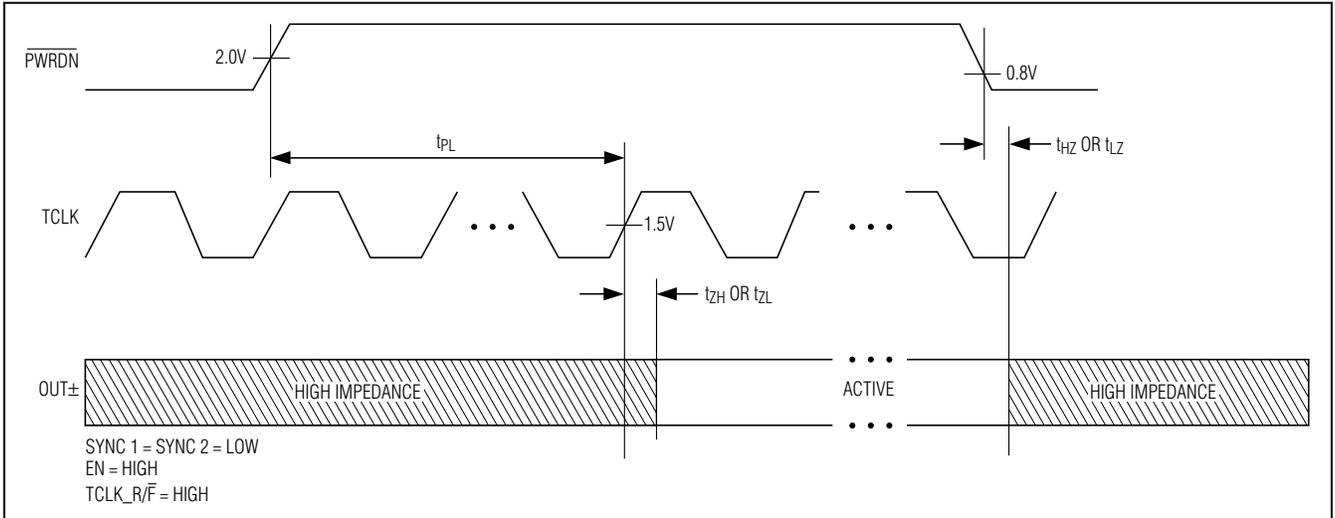
Figure 7. PLL Lock Time and PWRDN High-Impedance Delays
