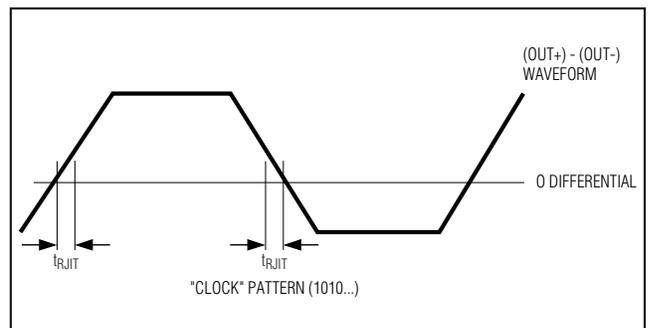
Figure 10. Definition of Random Jitter ( $t_{RJIT}$ )
