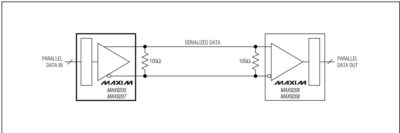
Figure 11. Double-Terminated Point-to-Point
