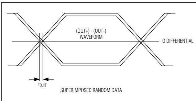
Figure 9. Definition of Deterministic Jitter ( $t_{DJIT}$ )
