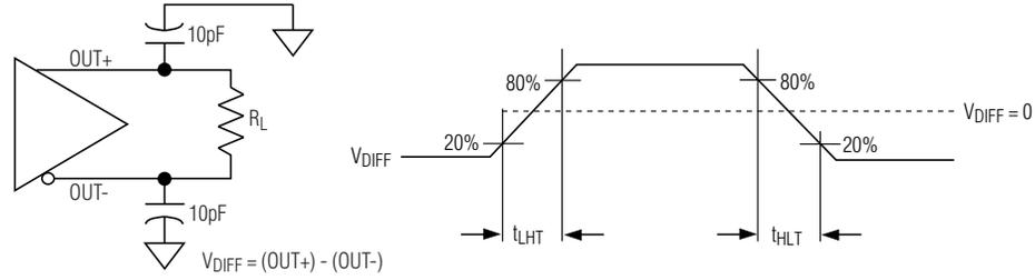
Figure 4. Output Load and Transition Times
