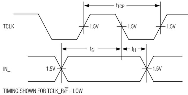
Figure 5. Data Input Setup and Hold Times
