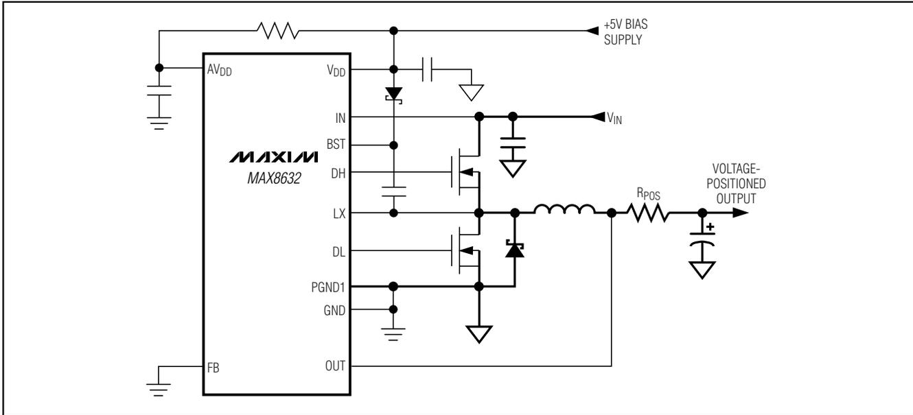
Figure 9. Voltage-Positioned Output
