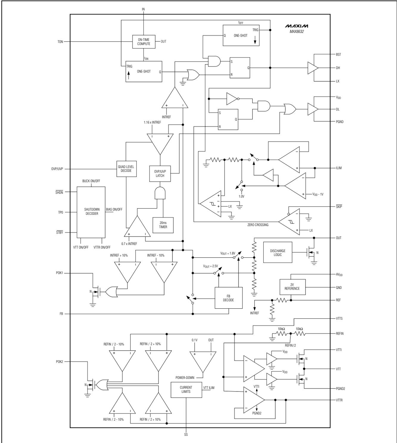
Figure 1. Functional Diagram
