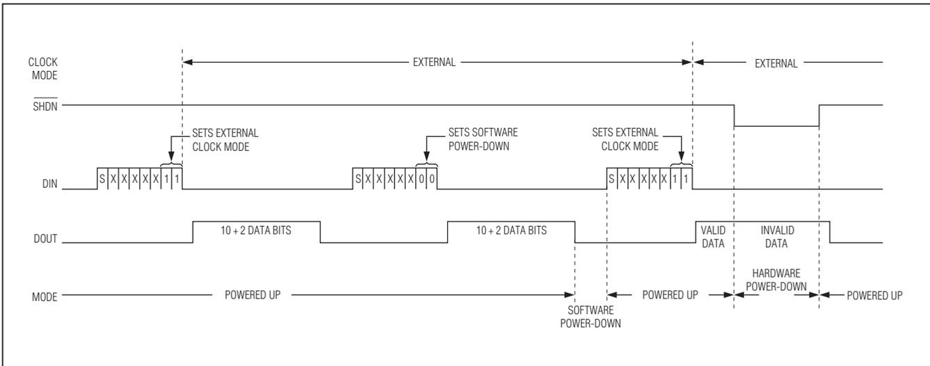
Figure 12a. Timing Diagram Power-Down Modes, External Clock
