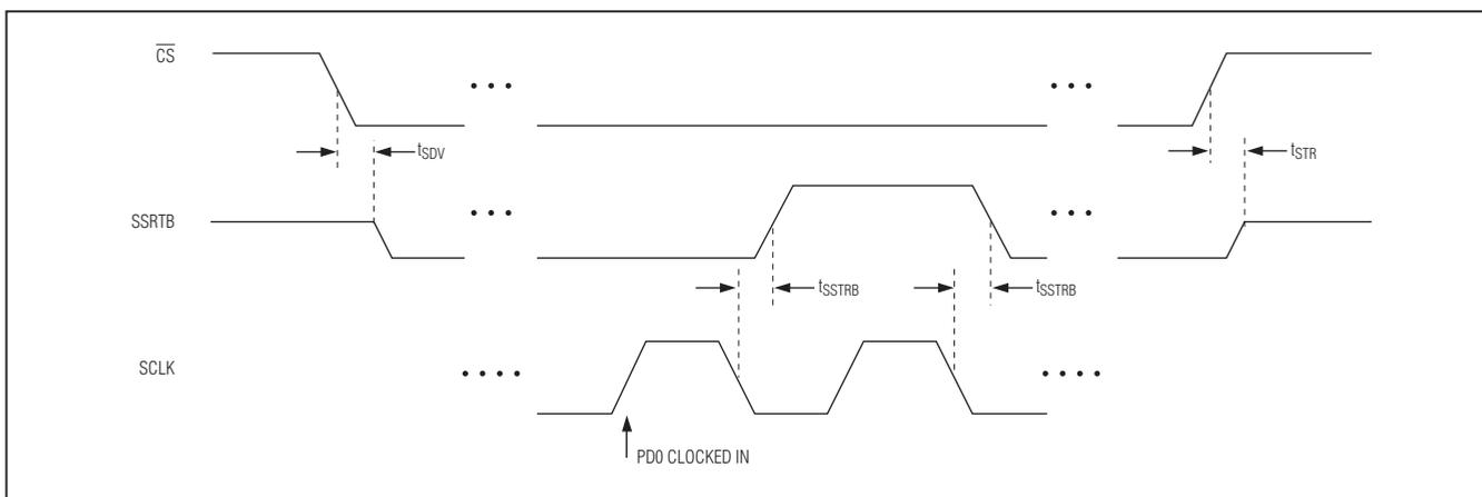
Figure 8. External Clock Mode SSTRB Detailed Timing
