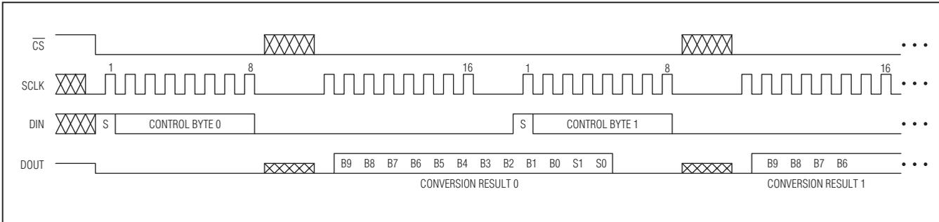
Figure 11b. External Clock Mode, 16 Clocks/Conversion Timing
