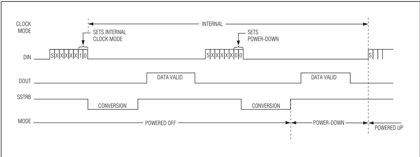
Figure 12b. Timing Diagram Power-Down Modes, Internal Clock
