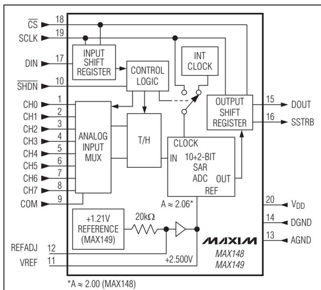
Figure 3. Block Diagram
