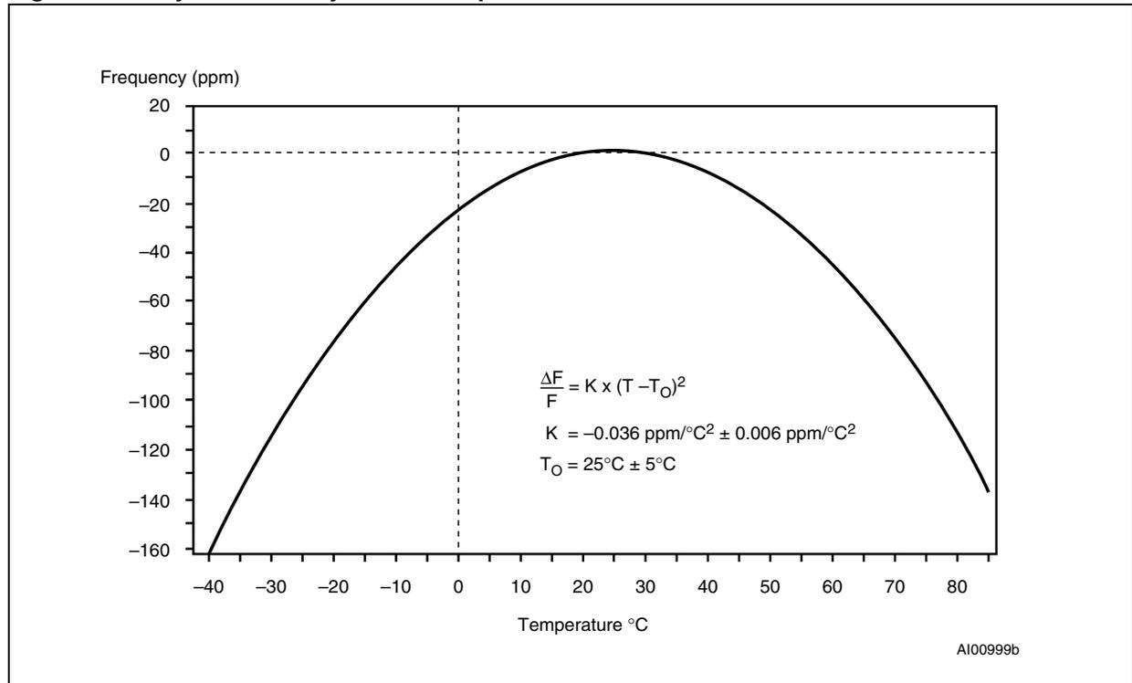
Figure 13. Clock calibration
