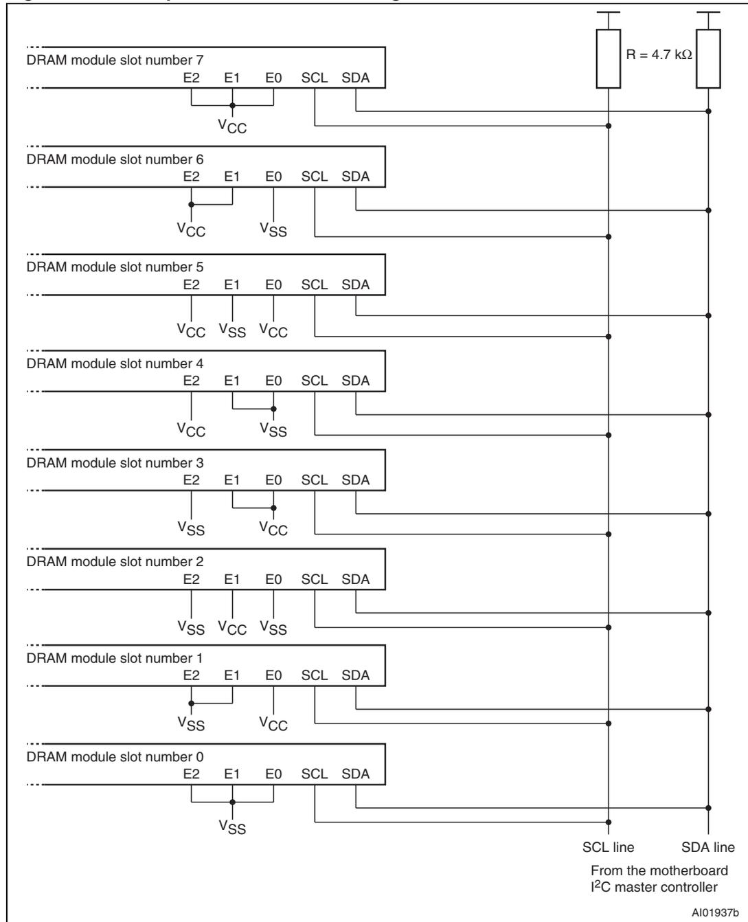
1. E0, E1 and E2 are wired at each DRAM module slot in a binary sequence for a maximum of 8 devices.
