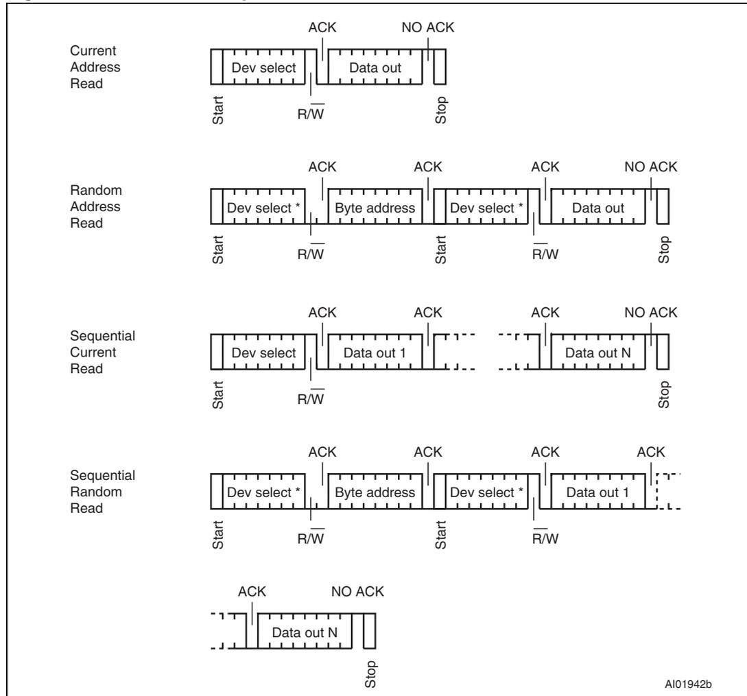
1. The seven most significant bits of the device select code of a Random Read (in the 1<sup>st</sup> and 3<sup>rd</sup> bytes) must be identical.
