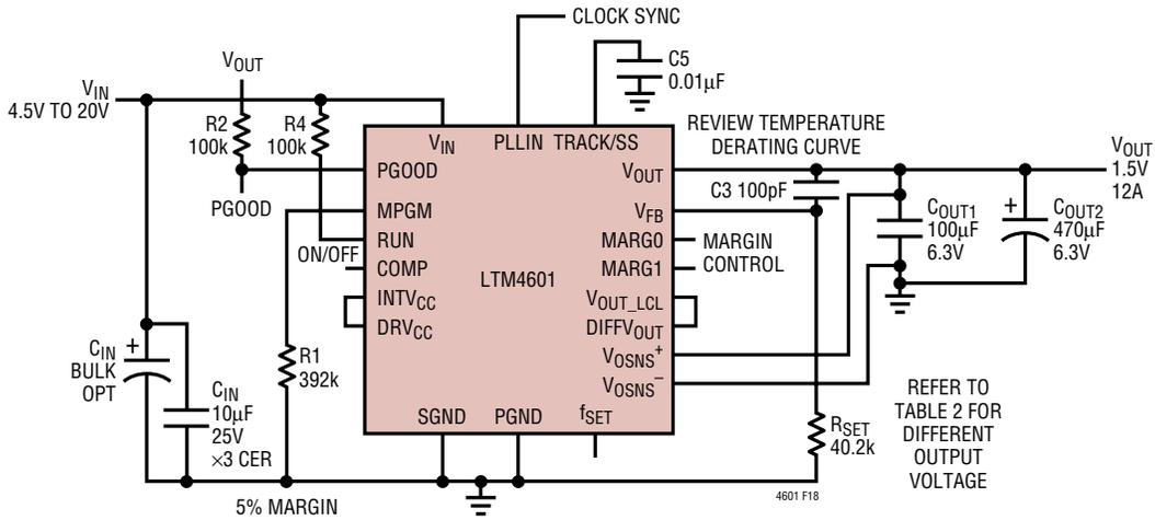
Figure 18. Typical 4.5V-20VIN, 1.5V at 12A Design
