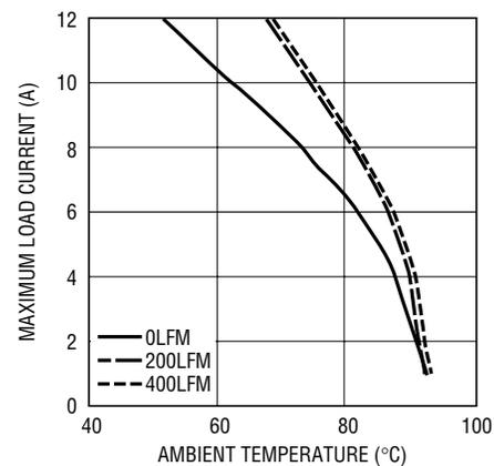
Figure 14. 12V<sub>IN</sub>, 3.3V<sub>OUT</sub>, BGA Heat Sink
