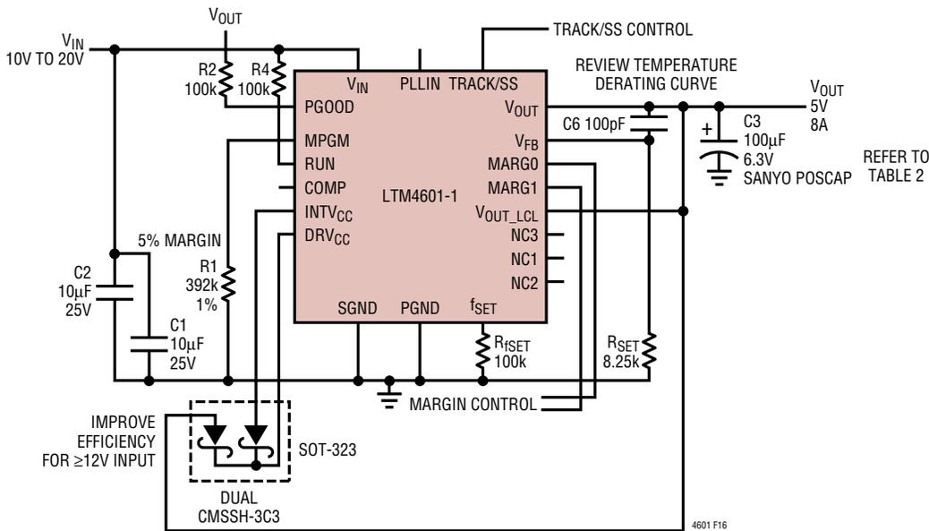
Figure 16. 5V at 8A Design Without Differential Amplifier
