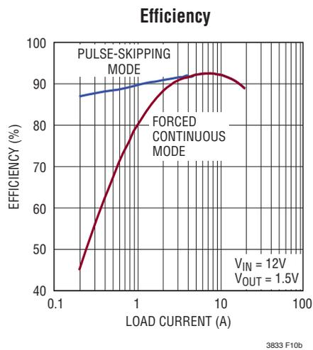
Figure 10. 1.5V, 20A, 300kHz High Current Step-Down Converter
