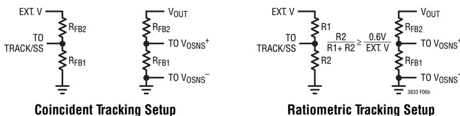
Figure 6b. Setup for Coincident and Ratiometric Tracking
