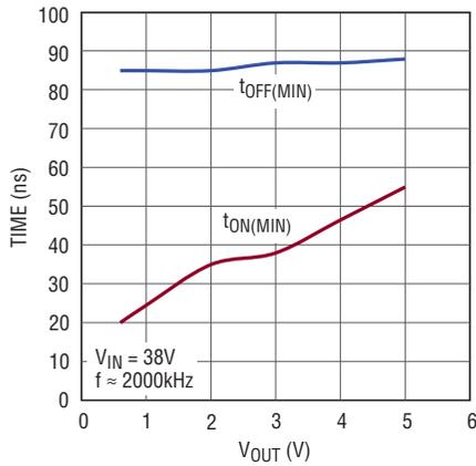
**$t_{ON(MIN)}$  and  $t_{OFF(MIN)}$  vs Voltage on  $V_{IN}$  Pin**
