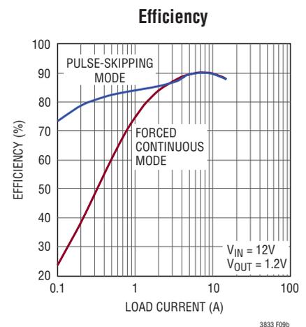
Figure 9. 1.2V, 15A, 350kHz Step-Down Converter
