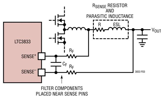
Figure 3. R<sub>SENSE</sub> Current Sensing
