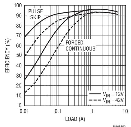
Figure 2. Efficiency in Pulse Skip/ Forced Continuous Modes
