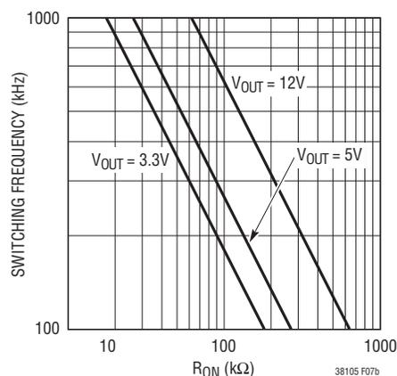
Figure 7b. Switching Frequency vs  $R_{ON}$  ( $V_{ON} = INTV_{CC}$ )
