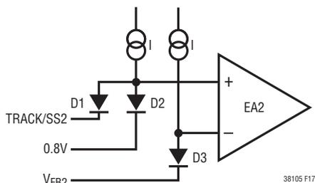
Figure 17. Equivalent Input Circuit of Error Amplifier
