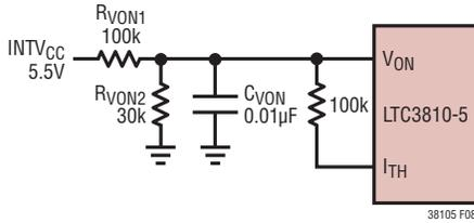
Figure 8. Correcting Frequency Shift with Load Current Changes
