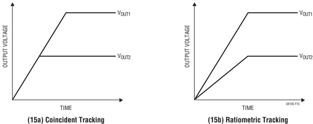
Figure 15. Two Different Modes of Output Voltage Tracking
