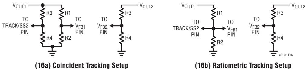
Figure 16. Setup for Coincident and Ratiometric Tracking
