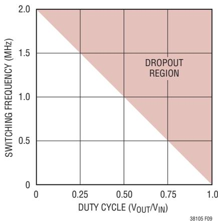
Figure 9. Maximum Switching Frequency vs Duty Cycle
