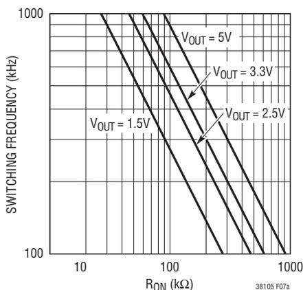
Figure 7a. Switching Frequency vs  $R_{ON}$  ( $V_{ON} = 0V$ )
