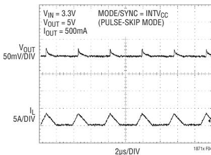
**Figure 4. LTC1871X Low Output Current Operation with Burst Mode Operation Disabled (MODE/SYNC = INTV<sub>CC</sub>)**
