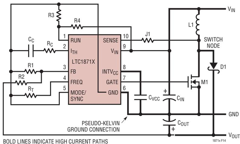
Figure 14. LTC1871X Boost Converter Layout Diagram
