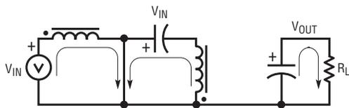
15b. Current Flow During Switch On-Time
