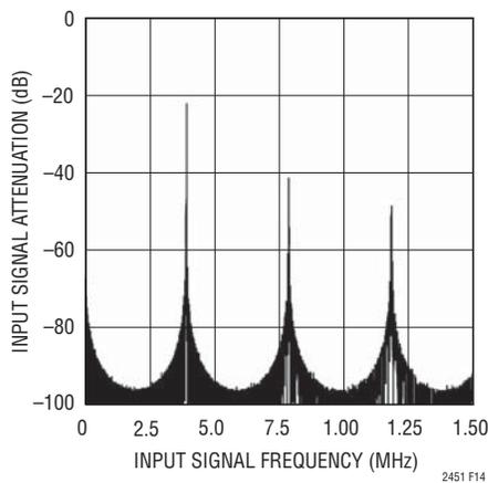
Figure 14. LTC2451 Input Signal Attenuation vs Frequency
