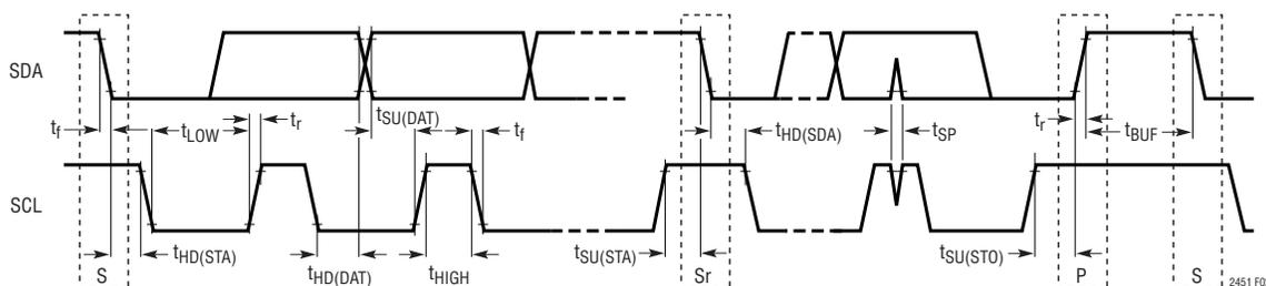
Figure 2. Definition of Timing for Fast/Standard Mode Devices on the I<sup>2</sup>C Bus
