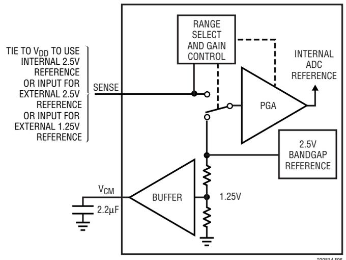
**Figure 6. Reference Circuit**
