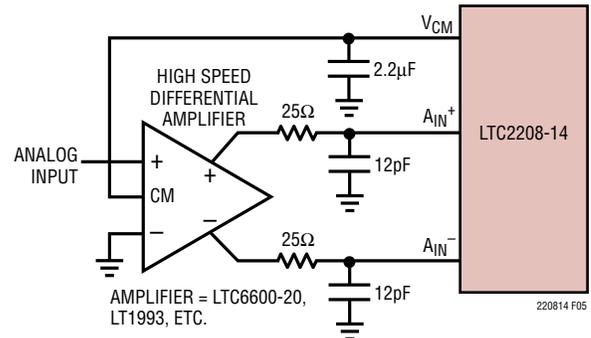
**Figure 5. DC Coupled Input with Differential Amplifier**
