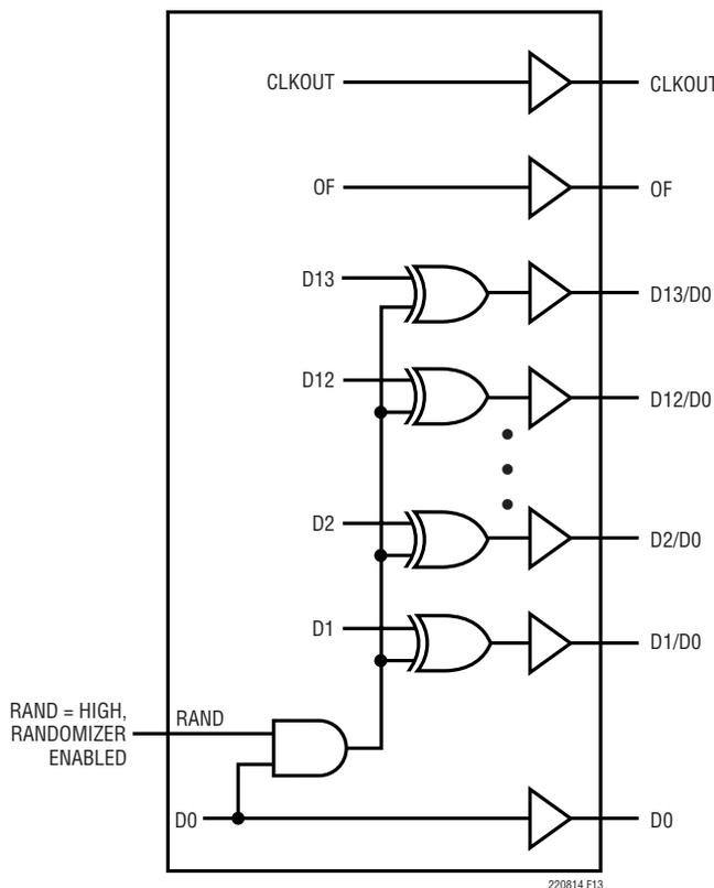
Figure 13. Functional Equivalent of Digital Output Randomizer
