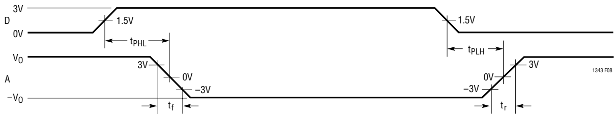
Figure 8. V.10, V.28 Driver Propagation Delays
