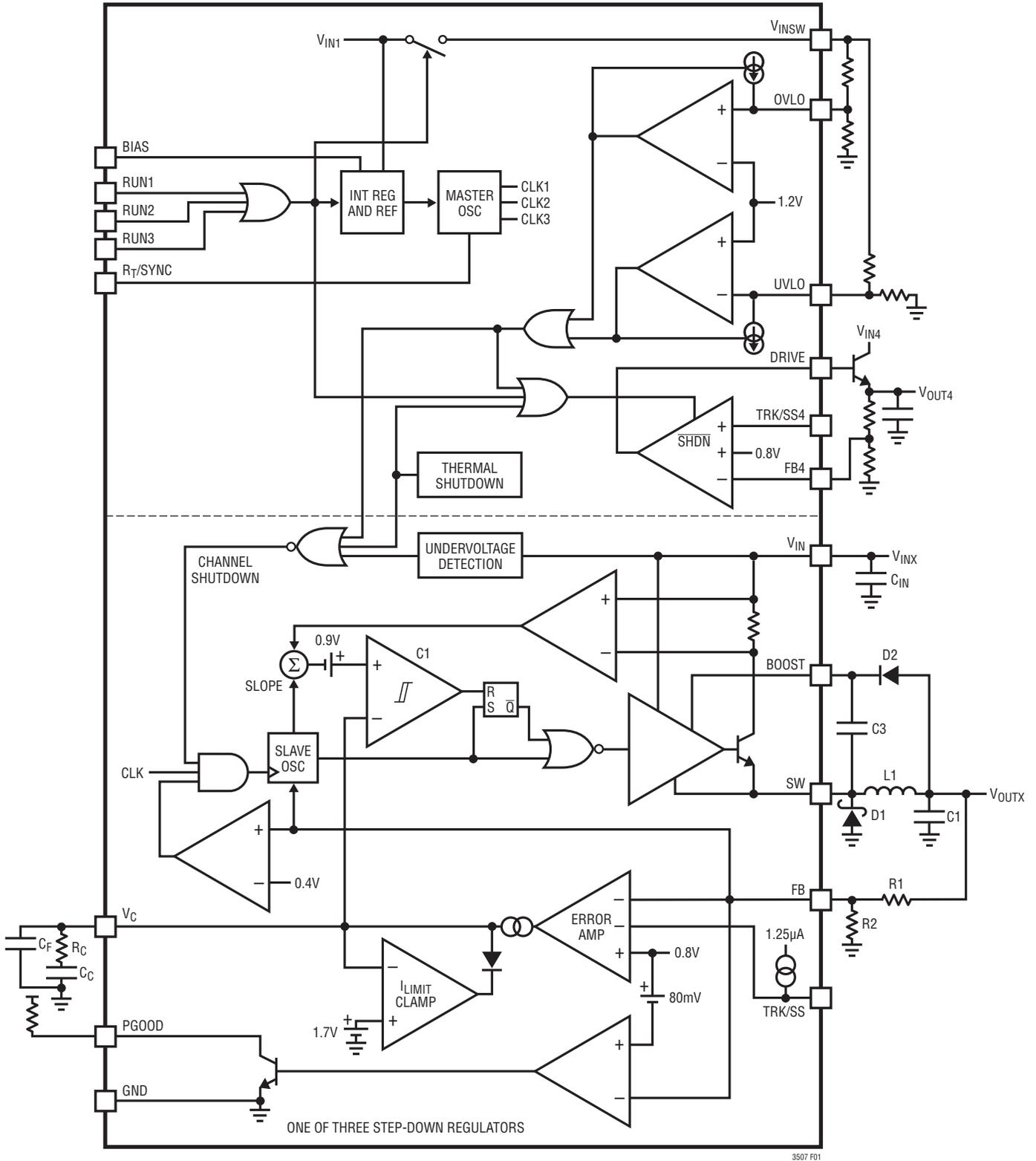
Figure 1. LT3507 Block Diagram with Typical External Components
