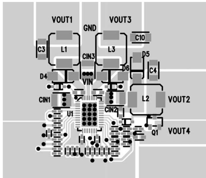
Figure 13. Power Path Components and Topside Layout
