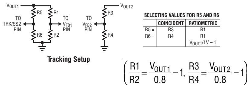
Figure 9. Setup for Coincident and Ratiometric Tracking
