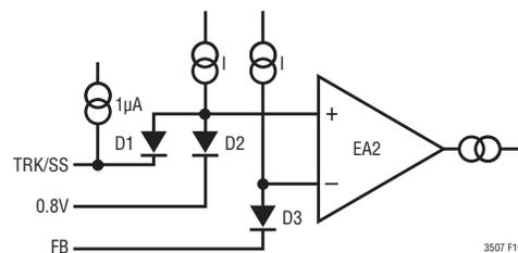
Figure 10. Equivalent Input Circuit of Error Amplifier
