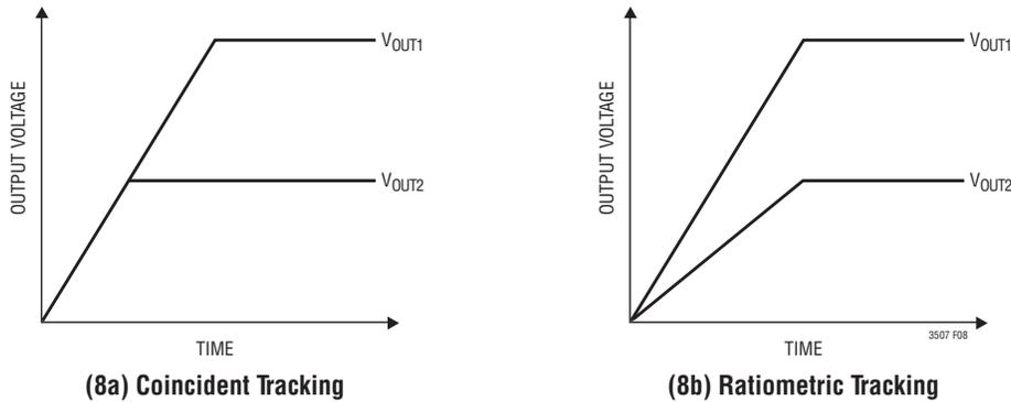
Figure 8. Two Different Modes of Output Voltage Tracking
