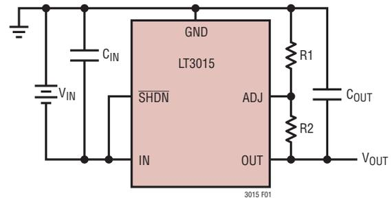
$$V_{OUT} = -1.22V \left( 1 + \frac{R_2}{R_1} \right) + (I_{ADJ})(R_2)$$
