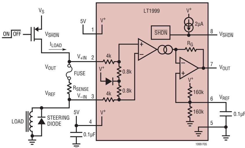
Figure 5. Using the LT1999 to Monitor a Fuse
