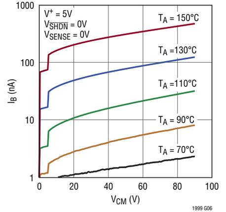
**Input Bias Current vs Input Common Mode**
