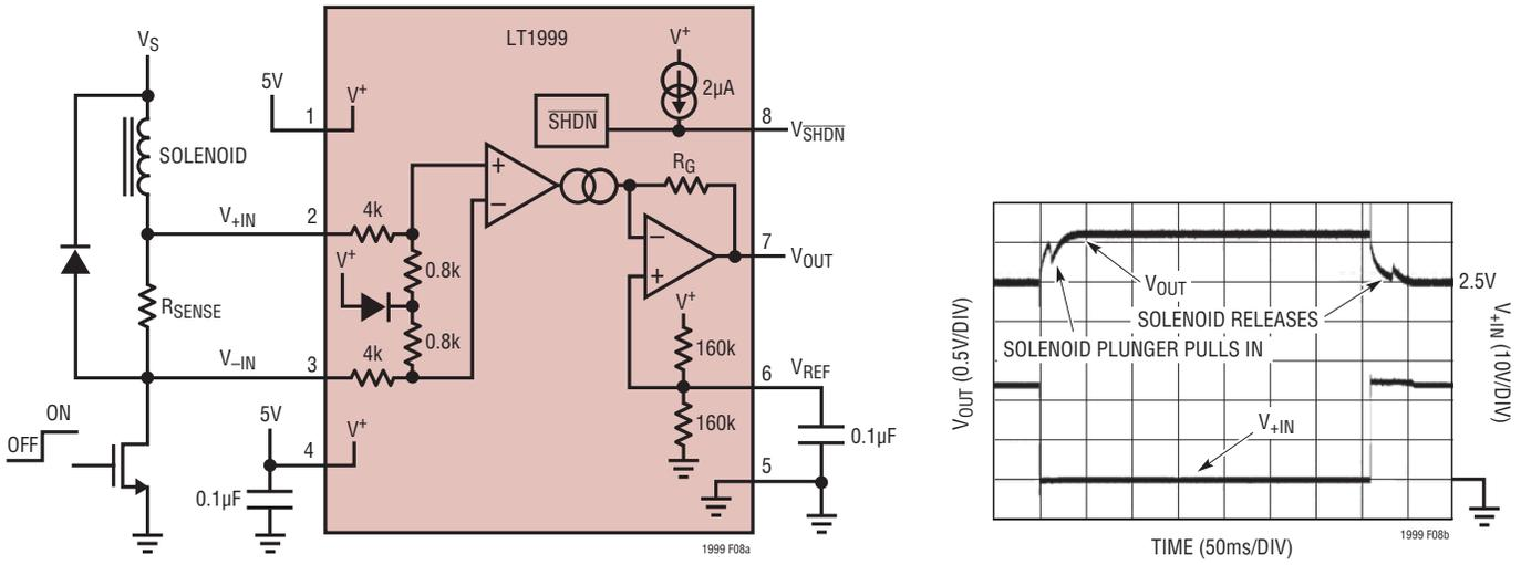
**Figure 8. Solenoid Current Monitor for Non-Grounded Solenoids. This Circuit Performs the Same Function as Figure 7 Except One End of the Solenoid Is Tied to  $V_S$ . The Common Mode Voltage of Inputs of the LT1999 Switch Between Ground and One Diode Drop Above  $V_S$**
