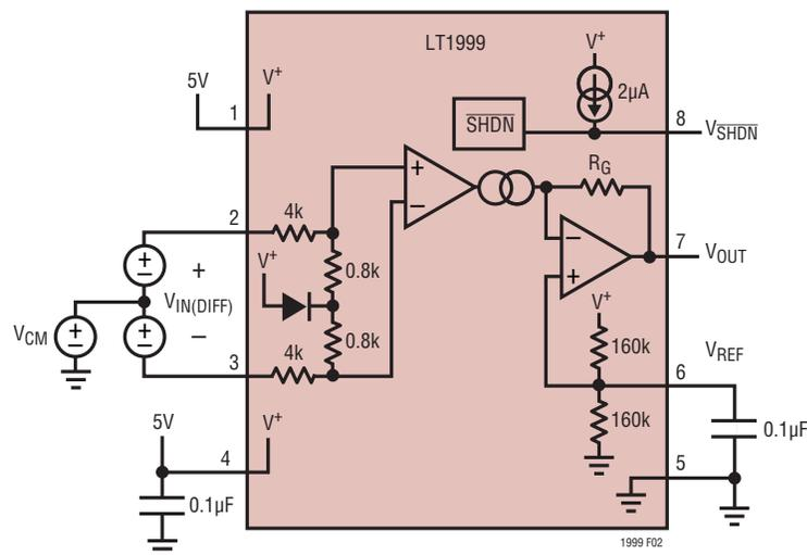
Figure 2. Test Circuit
