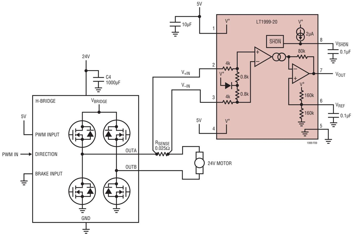
Figure 9. Armature Current Monitor for DC Motor Applications
