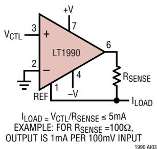
**Boosted Bidirectional Controlled Current Source**
