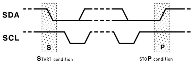
Figure 3. I<sup>2</sup>C START and STOP Conditions
