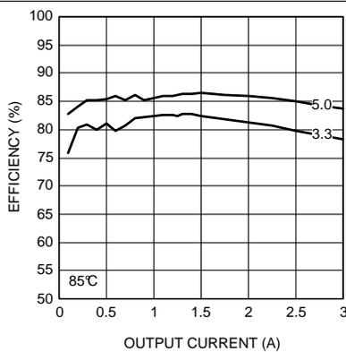
Figure 17. Efficiency 36-V Input at 85°C
