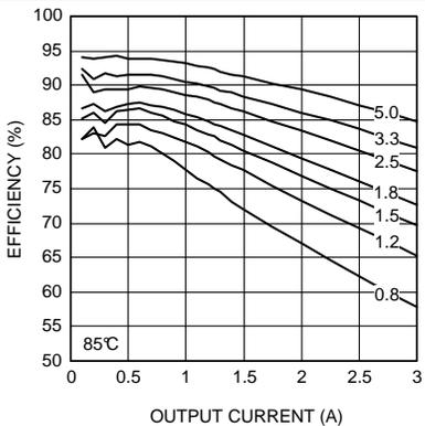
Figure 11. Efficiency 8-V Input at 85°C
