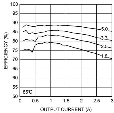
Figure 15. Efficiency 24-V Input at 85°C
