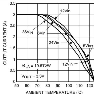
Figure 22. Thermal Derating  $V_{OUT} = 3.3\text{ V}$
