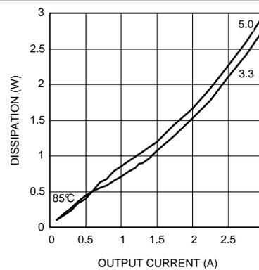
Figure 18. Dissipation 36-V Input at 85°C
