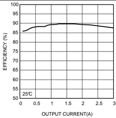
Figure 27. Efficiency  $V_{IN} = 24\text{ V}$   $V_{OUT} = 5.0\text{ V}$
