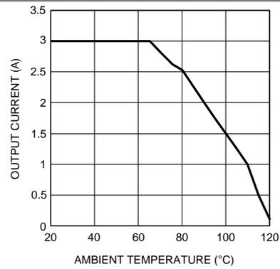
Figure 28. Thermal Derating Curve
