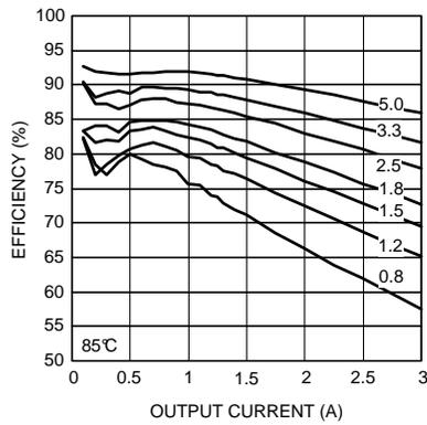
Figure 13. Efficiency 12-V Input at 85°C
