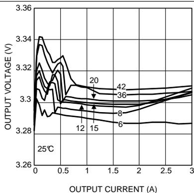
Figure 19. Line and Load Regulation at 25°C
