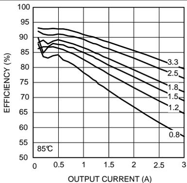
Figure 9. Efficiency 6-V Input at 85°C
