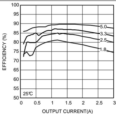
**Figure 5. Efficiency 24-V Input at 25°C**
