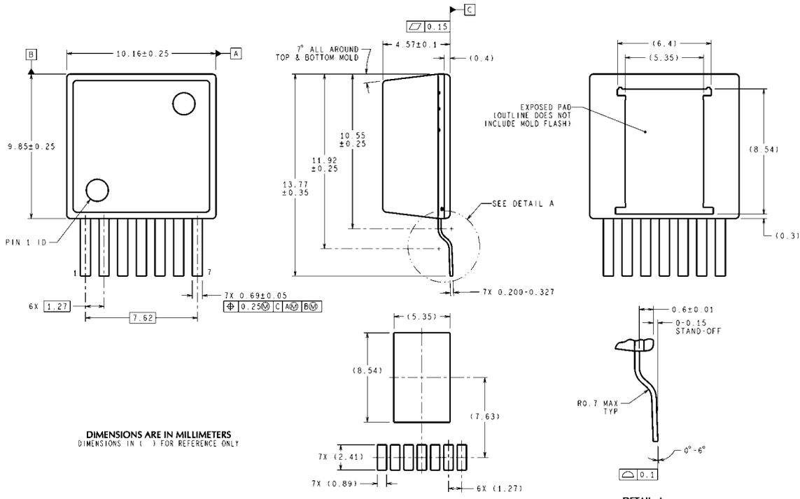
DIMENSIONS ARE IN MILLIMETERS
