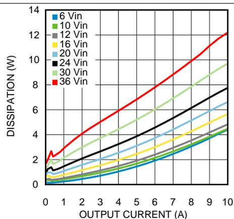
Figure 24. Dissipation 1.5-V Output at 85°C
