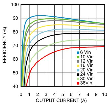
Figure 5. Efficiency 2.5-V Output at 25°C
