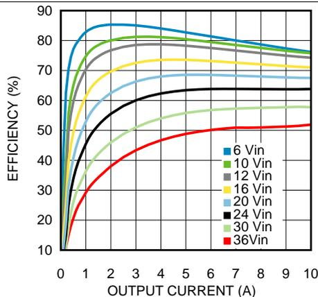
Figure 11. Efficiency 1.2-V Output at 25°C
