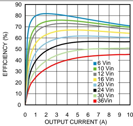
Figure 27. Efficiency 1-V Output at 85°C
