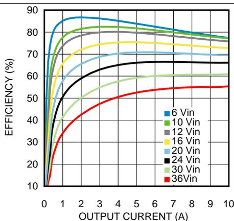
Figure 23. Efficiency 1.5-V Output at 85°C
