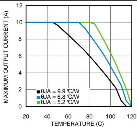
$V_{IN} = 24\text{ V}, V_{OUT} = 5\text{ V}$
