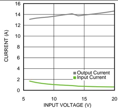
**Figure 42. Short Circuit Current vs Input Voltage**
