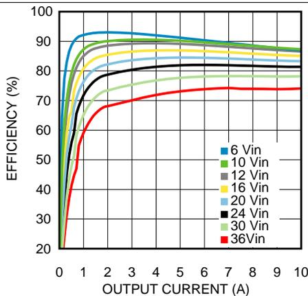
Figure 17. Efficiency 3.3-V Output at 85°C
