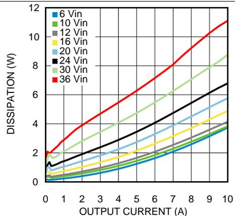
Figure 12. Dissipation 1.2-V Output at 25°C
