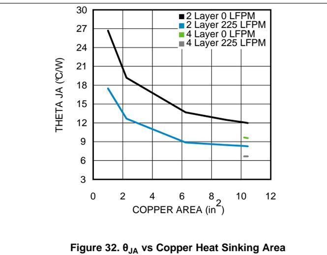
Figure 32.  $\theta_{JA}$  vs Copper Heat Sinking Area
