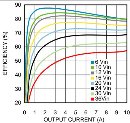
Figure 9. Efficiency 1.5-V Output at 25°C
