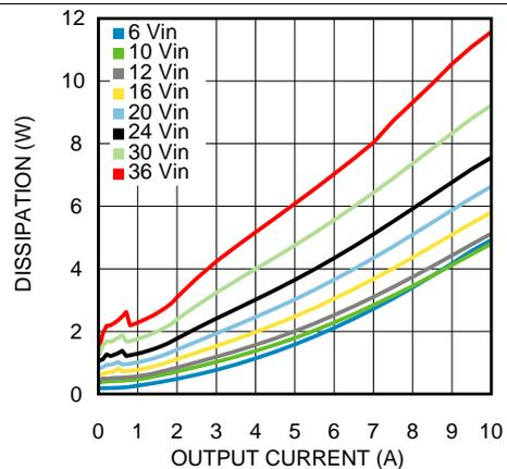
Figure 18. Dissipation 3.3-V Output at 85°C
