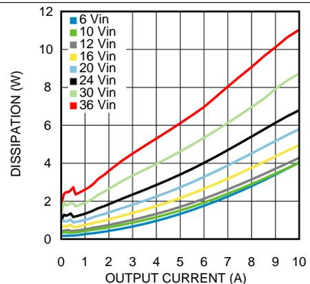
Figure 6. Dissipation 2.5-V Output at 25°C
