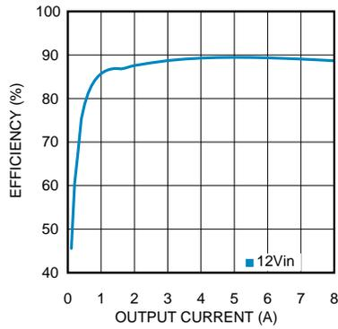
$V_{IN} = 12\text{ V}$ ,  $V_{OUT} = 3.3\text{ V}$
