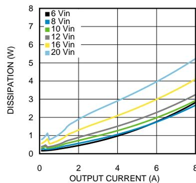
Figure 6. Dissipation 2.5-V Output at 25°C
