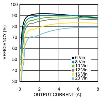
Figure 5. Efficiency 2.5-V Output at 25°C
