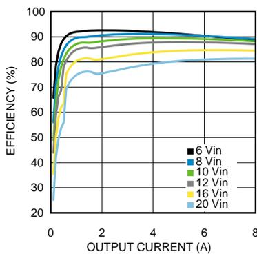
Figure 17. Efficiency 3.3-V Output at 85°C
