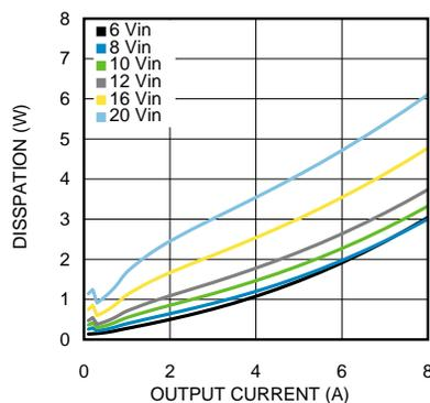
Figure 24. Dissipation 1.5-V Output at 85°C
