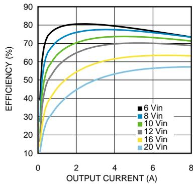
Figure 27. Efficiency 1-V Output at 85°C
