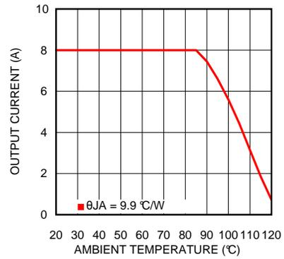
$V_{IN} = 12\text{ V}$ ,  $V_{OUT} = 3.3\text{ V}$
