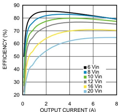
Figure 11. Efficiency 1.2-V Output at 25°C
