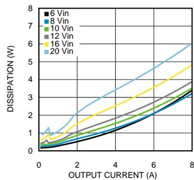
Figure 18. Dissipation 3.3-V Output at 85°C
