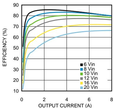
Figure 23. Efficiency 1.5-V Output at 85°C
