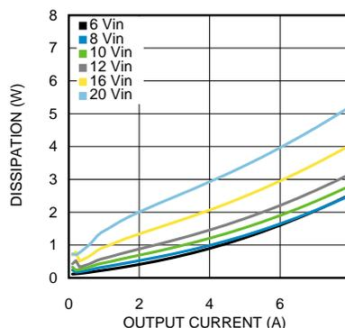
Figure 12. Dissipation 1.2-V Output at 25°C
