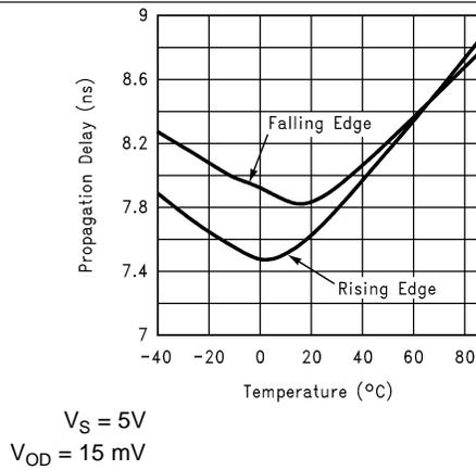
Figure 9. Propagation Delay vs. Temperature
