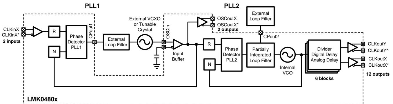
Figure 39. Simplified Functional Block Diagram for Dual-Loop Mode
