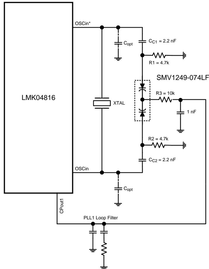
Figure 37. Reference Design Circuit for Crystal Oscillator Option
