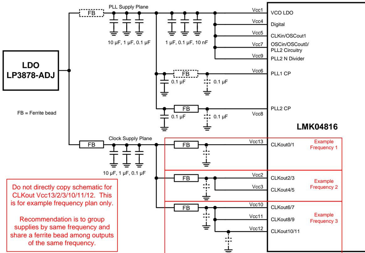
Figure 42. Example Application – Power System Schematic
