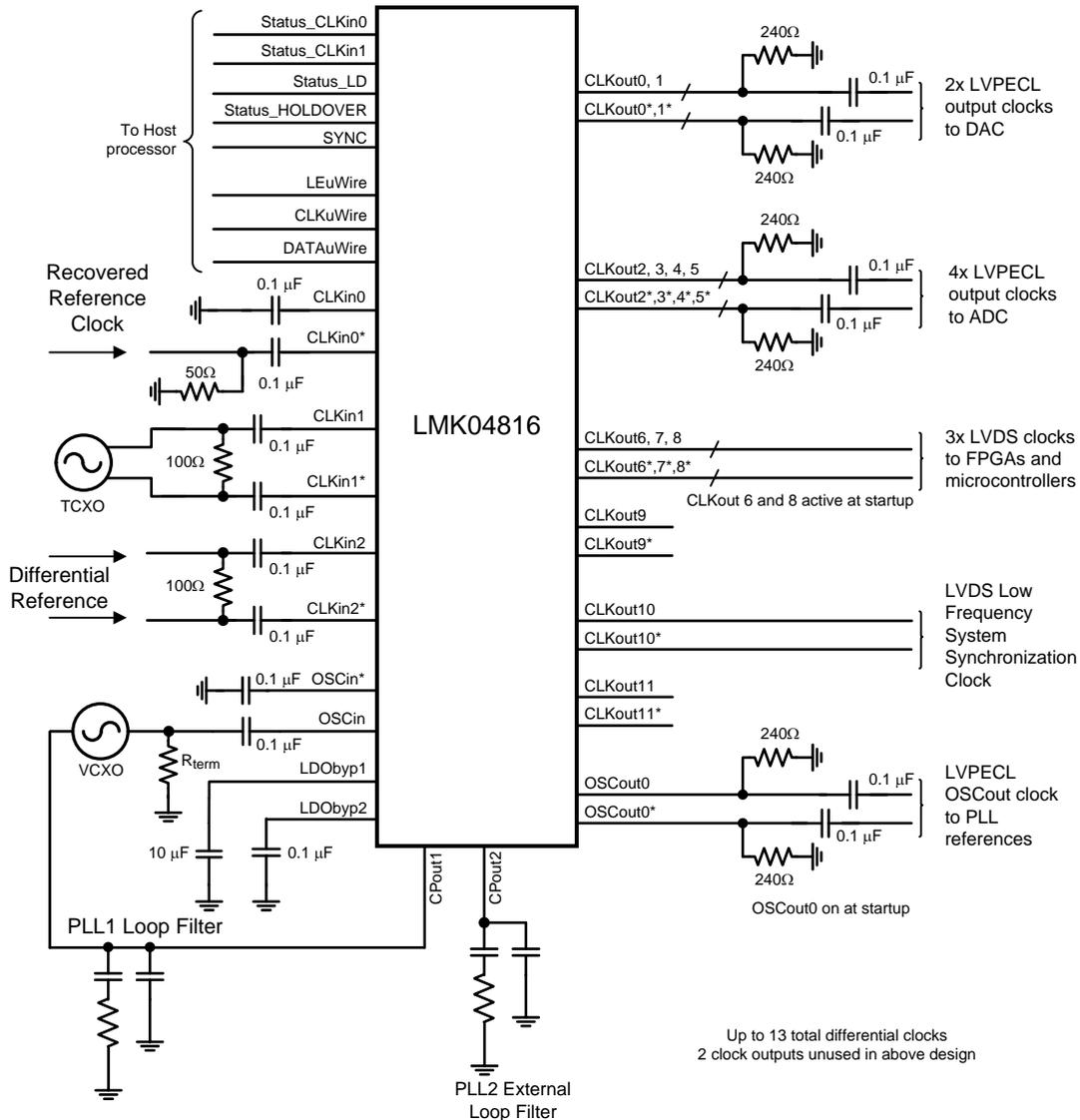
Figure 41. Example Application – System Schematic Except for Power
