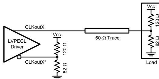
Figure 35. Single-Ended LVPECL Operation, DC Coupling, Thevenin Equivalent
