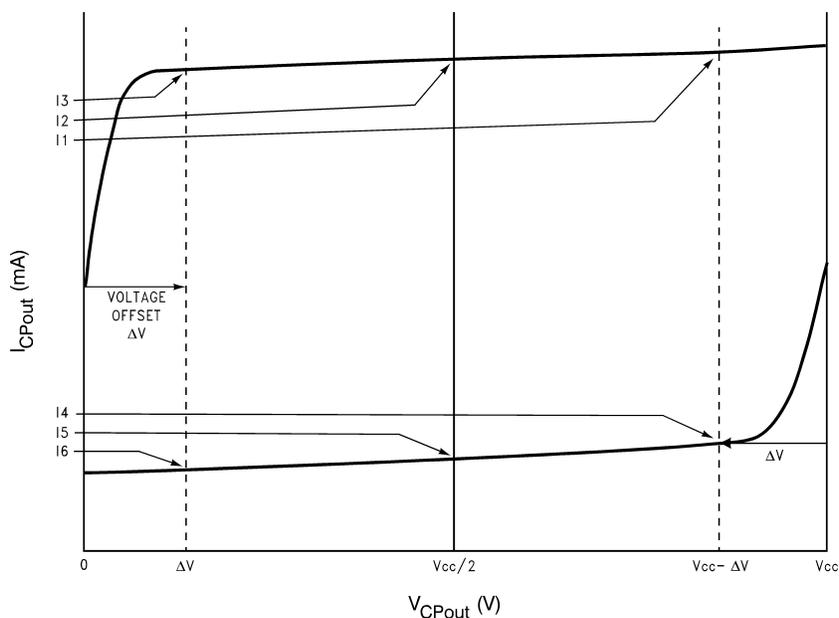
**Figure 4. Charge-Pump Current**
