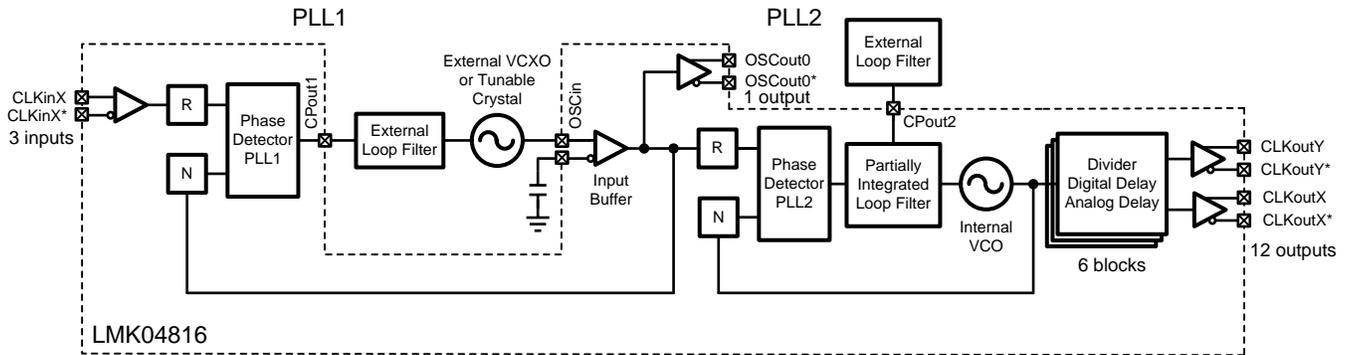
Figure 17. Simplified Functional Block Diagram for Dual-Loop Mode
