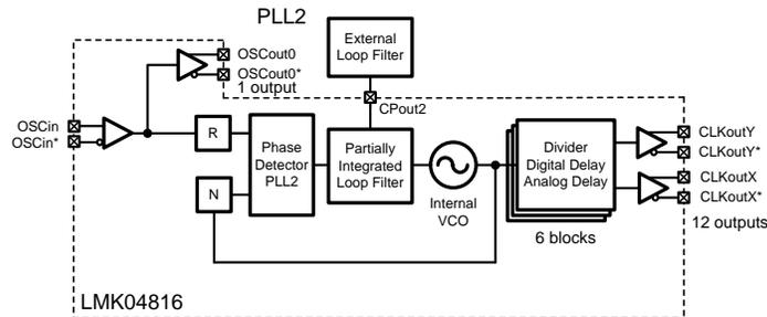
Figure 19. Simplified Functional Block Diagram for Single-Loop Mode
