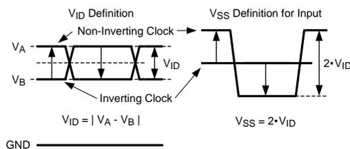
Figure 5. Two Different Definitions for Differential Input Signals
