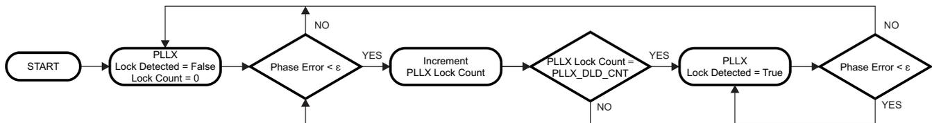
**Figure 12. Digital Lock Detect Flowchart**
