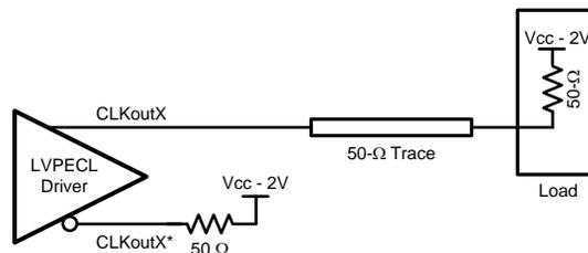
Figure 34. Single-Ended LVPECL Operation, DC Coupling
