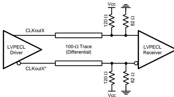
Figure 30. Differential LVPECL Operation, DC Coupling, Thevenin Equivalent
