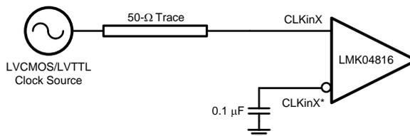
Figure 27. DC-Coupled LVCMOS and LVTTTL Reference Clock
