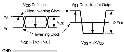
Figure 6. Two Different Definitions for Differential Output Signals
