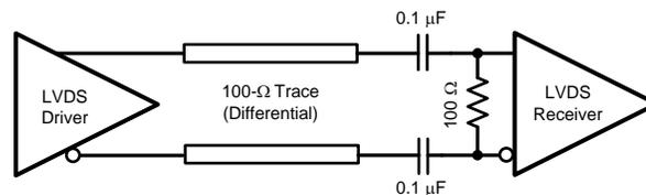
Figure 32. LVDS Termination for a Self-Biased Receiver
