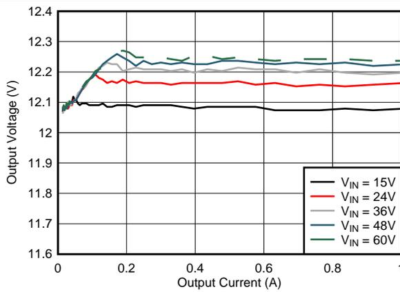
Figure 6. Load and Line Regulation Performance
