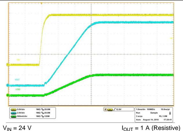
Figure 9. Full-Load Start-up with VIN
