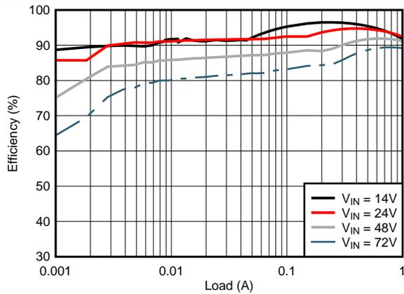
Figure 4. Conversion Efficiency (Log Scale)
