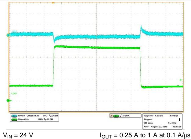
Figure 7. Load Step Response
