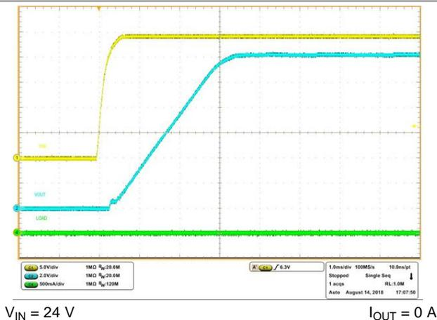
Figure 8. No-Load Start-up with VIN
