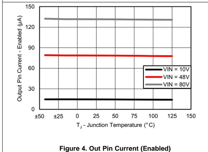
Figure 4. Out Pin Current (Enabled)
