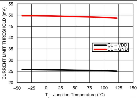
Figure 16. Current Limit Threshold
