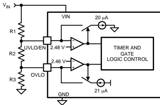
**Figure 30. UVLO And OVLO Thresholds Set By R1-R3**
