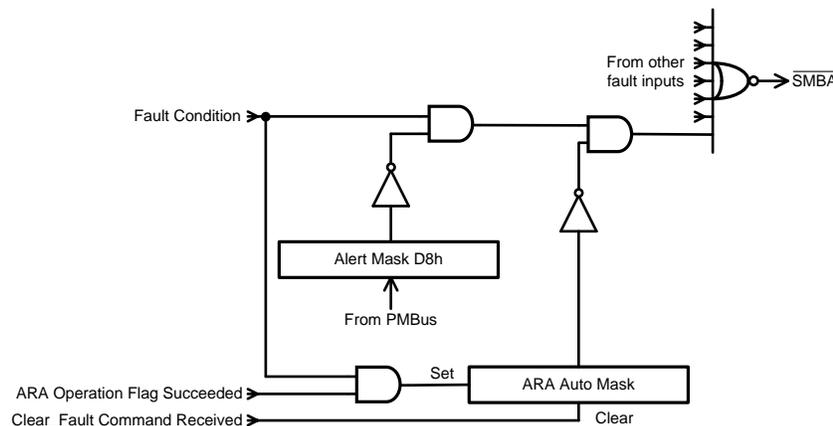
**Figure 27. Typical Flow Schematic for SMBA Fault**
