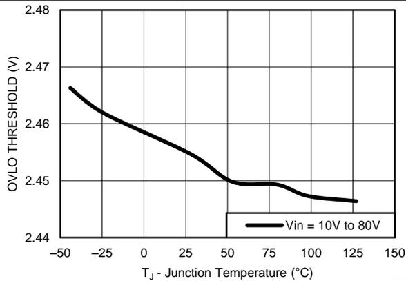
Figure 14. OVLO Threshold
