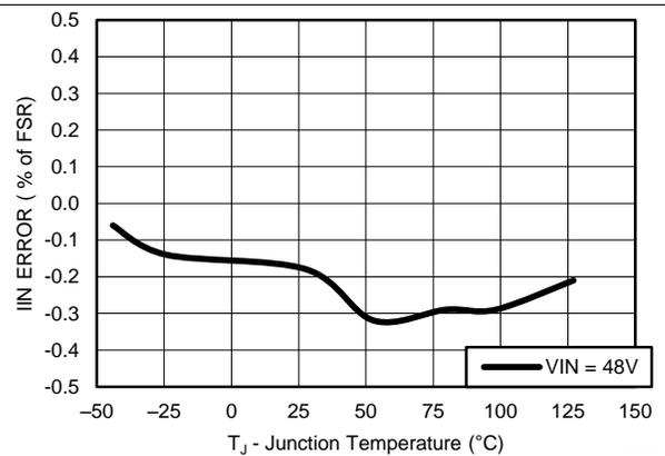
Figure 19. IIN Measurement Accuracy
