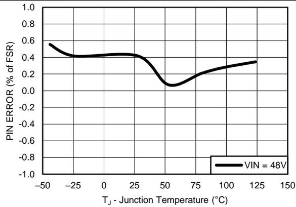
Figure 20. Pin Measurement Accuracy ( $V_{IN} - \text{Sense} = 50\text{ mV}$ )
