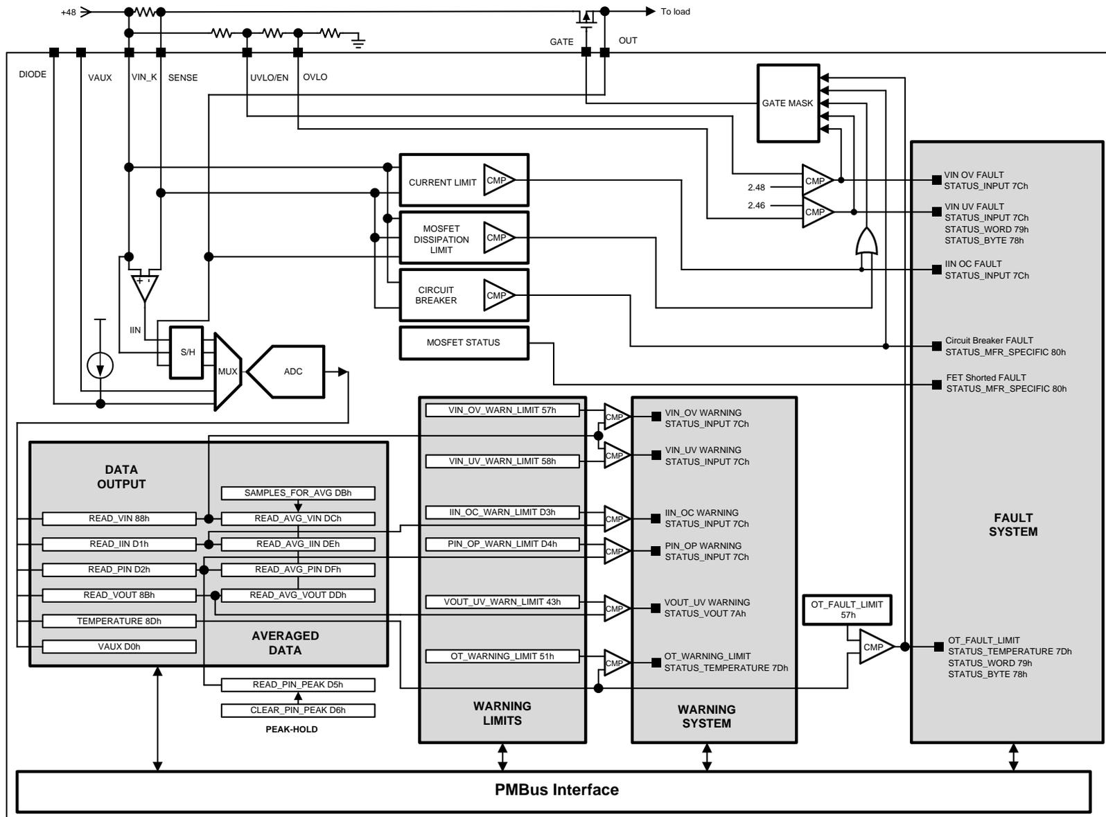
Figure 26. Command / Register and Alert Flow Diagram
