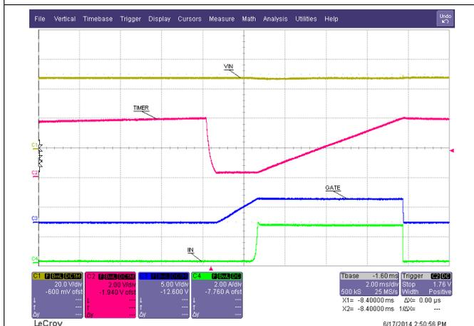
Figure 41. Start-Up into Short Circuit
