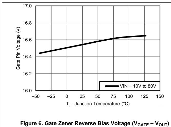
Figure 6. Gate Zener Reverse Bias Voltage ( $V_{GATE} - V_{OUT}$ )
