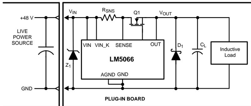
Figure 36. Output Diode Required for Inductive Loads
