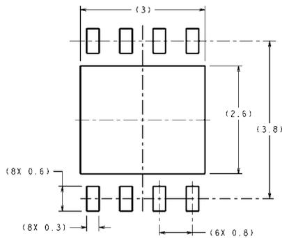
DIMENSIONS ARE IN MILLIMETERS
