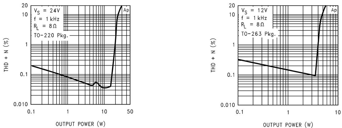
Figure 44. THD+N vs  $P_{OUT}$  for Bridge-Mode Application
