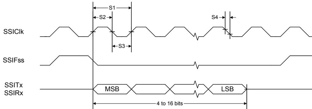
Figure 24-13. SSI Timing for MICROWIRE Frame Format (FRF=10), Single Transfer
