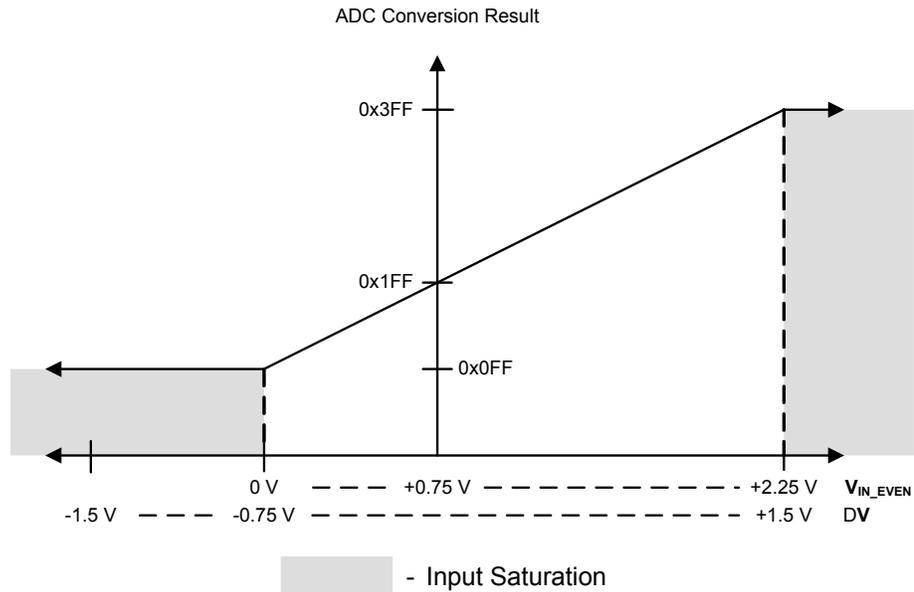
Figure 12-4. Differential Sampling Range,  $V_{IN\_ODD} = 2.25\text{ V}$
