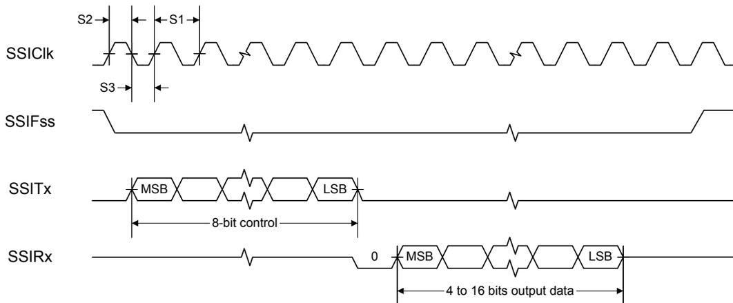
Figure 24-14. SSI Timing for SPI Frame Format (FRF=00), with SPH=1
