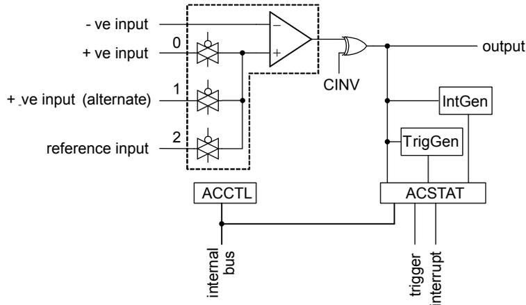
A comparator is configured through two status/control registers (**ACCTL** and **ACSTAT**). The internal reference is configured through one control register (**ACREFCTL**). Interrupt status and control is configured through three registers (**ACMIS**, **ACRIS**, and **ACINTEN**).
