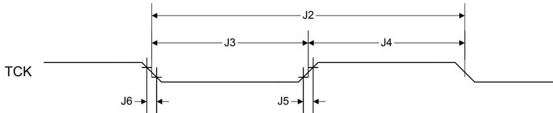
Figure 24-3. JTAG Test Access Port (TAP) Timing
