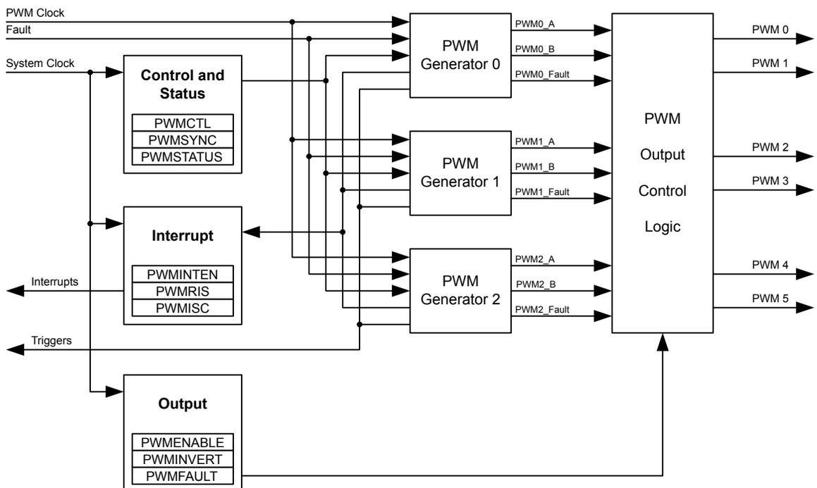
Figure 19-2. PWM Module Block Diagram
