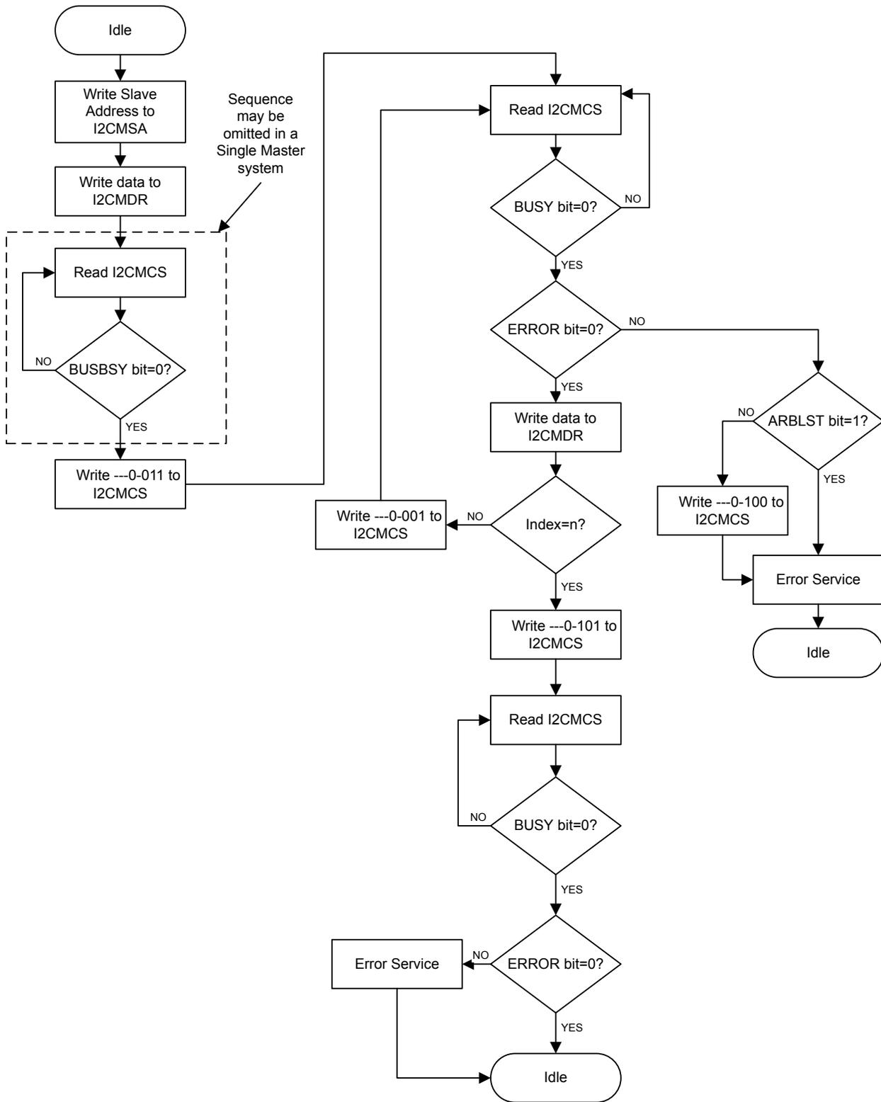
Figure 15-10. Master Burst RECEIVE
