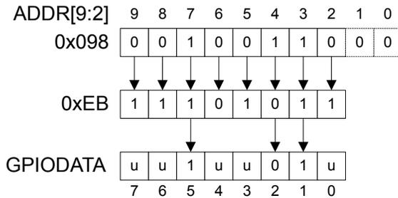
During a read, if the address bit associated with the data bit is set to 1, the value is read. If the address bit associated with the data bit is set to 0, it is read as a zero, regardless of its actual value. For example, reading address **GPIODATA** + 0x0C4 yields as shown in Figure 9-3 on page 188.
