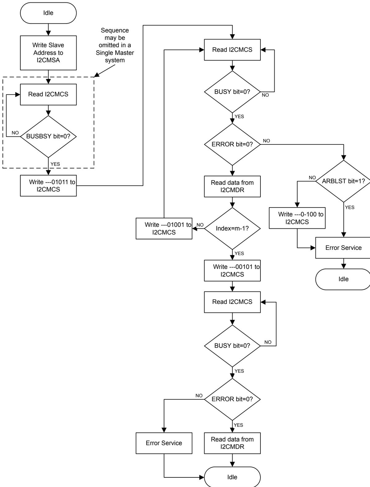
Figure 15-11. Master Burst RECEIVE after Burst SEND
