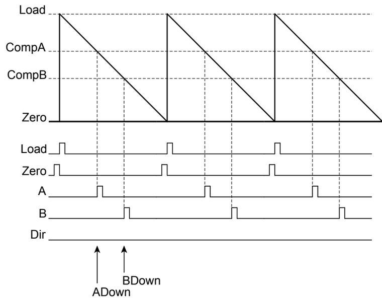
**Figure 19-4. PWM Count-Up/Down Mode**
