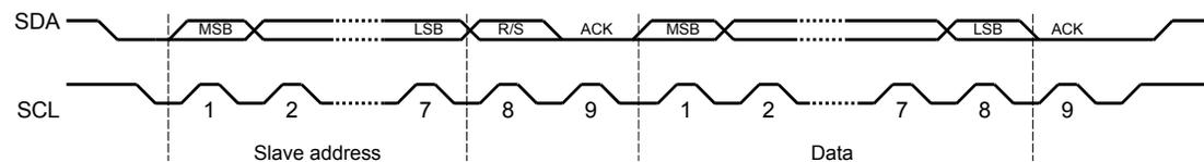
The first seven bits of the first byte make up the slave address (see Figure 15-5 on page 405). The eighth bit determines the direction of the message. A zero in the R/S position of the first byte means that the master will write (send) data to the selected slave, and a one in this position means that the master will receive data from the slave.
