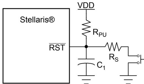
$$\text{Typical } R_{PU} = 10 \text{ k}\Omega$$
