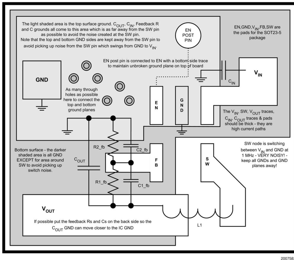
FIGURE 6. Board Layout Design Rules for the LM3670
