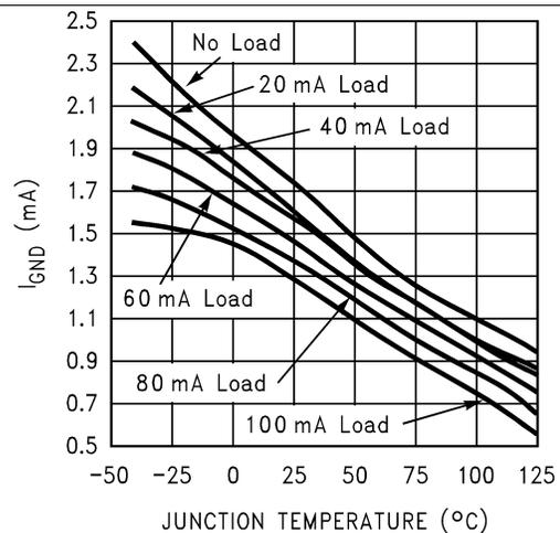
Figure 6. Ground Pin Current vs Junction Temperature
