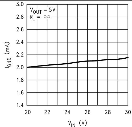
Figure 4. Ground Pin Current vs Input Voltage
