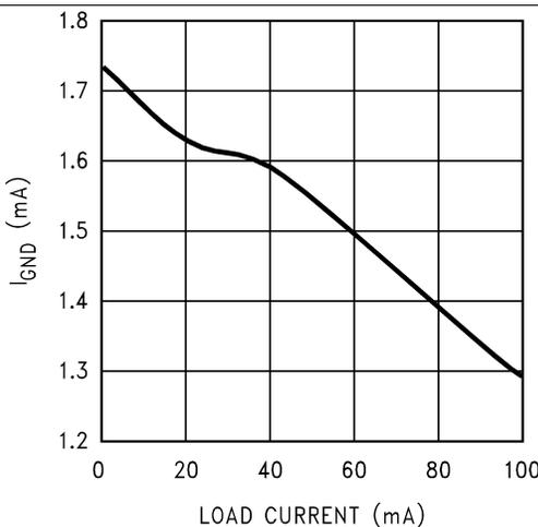
Figure 5. Ground Pin Current vs Load Current
