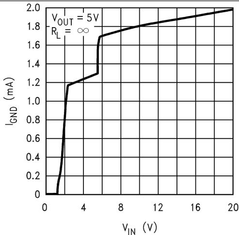
Figure 3. Ground Pin Current vs Input Voltage
