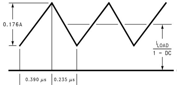
Figure 14. 10 µH Inductor Current, 5 V – 12 V Boost
