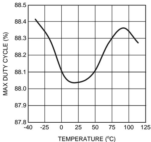
**Figure 3. Max. Duty Cycle vs Temperature**
