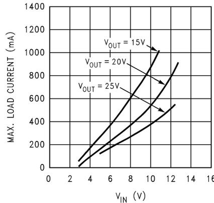
Figure 16. Max. Load Current vs V<sub>IN</sub>
