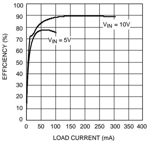
Figure 11. Efficiency vs Load Current ( $V_{OUT} = 25\text{ V}$ )
