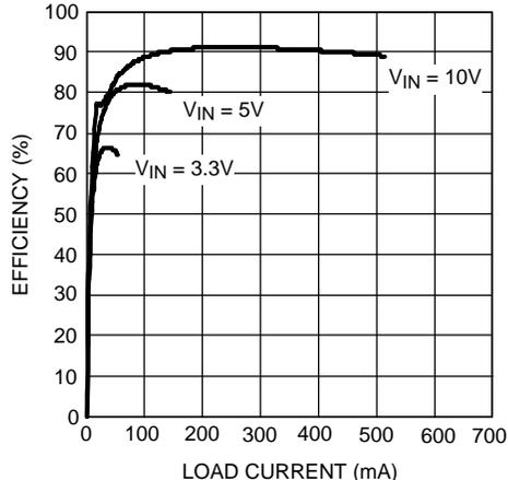
Figure 10. Efficiency vs Load Current ( $V_{OUT} = 20\text{ V}$ )
