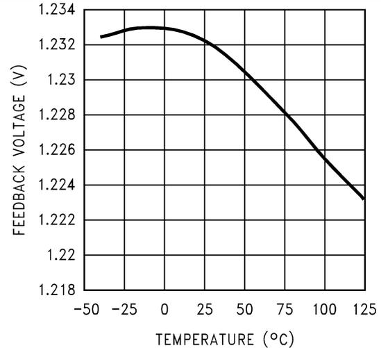
**Figure 4. Feedback Voltage vs Temperature**
