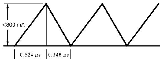
Figure 17. Discontinuous Design, 5 V – 12 V Boost
