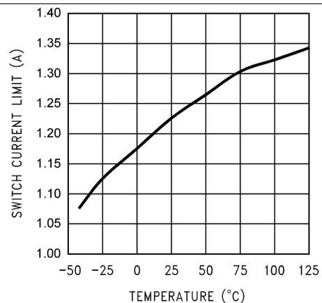
**Figure 6. Current Limit vs Temperature**
