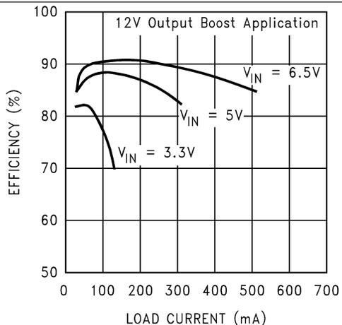
Figure 8. Efficiency vs Load Current ( $V_{OUT} = 12\text{ V}$ )
