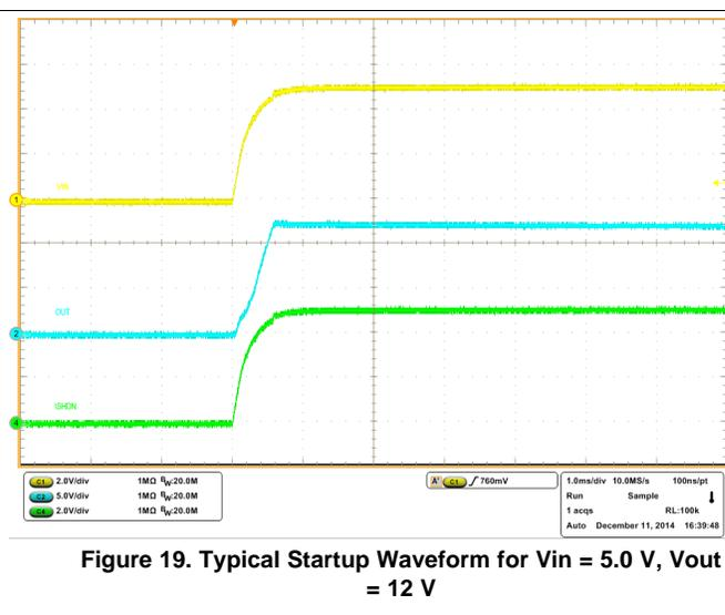
Figure 19. Typical Startup Waveform for  $V_{in} = 5.0 \text{ V}$ ,  $V_{out} = 12 \text{ V}$
