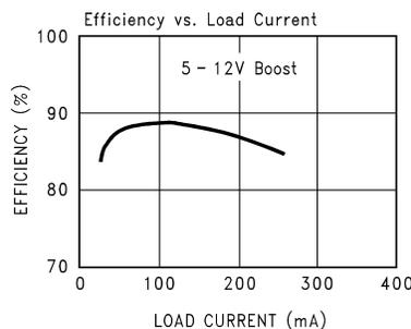
Figure 13. Efficiency vs. Load Current
