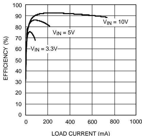
Figure 9. Efficiency vs Load Current ( $V_{OUT} = 15\text{ V}$ )
