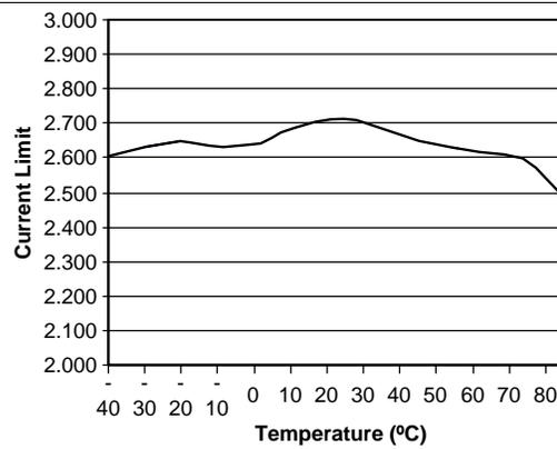
Figure 6. Typical Current Limit vs Temperature
