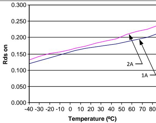
Figure 5. Typical  $R_{DS(ON)}$  vs Temperature
