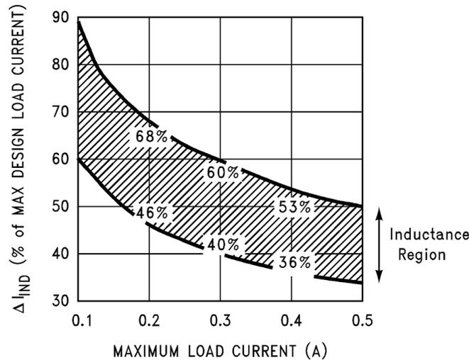
**Figure 19. Inductor Ripple Current ( $\Delta I_{IND}$ ) Range**
