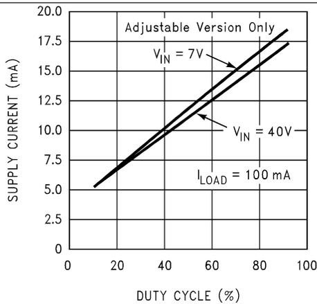
Figure 11. Supply Current vs Duty Cycle
