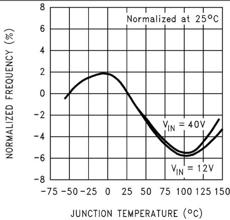
Figure 7. Oscillator Frequency
