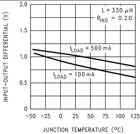
Figure 3. Dropout Voltage
