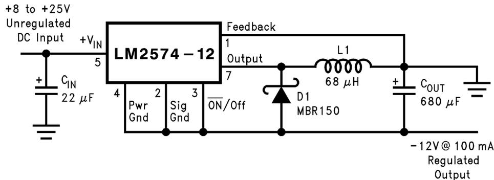
**Note:** Pin numbers are for the 8-pin PDIP package.
