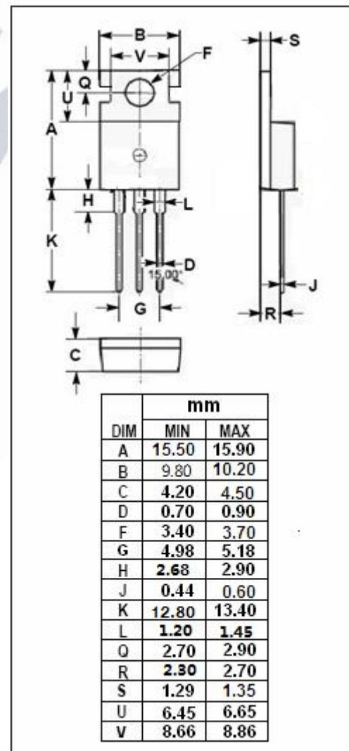
**isc Three Terminal Negative Voltage Regulator****L7905CV****• ELECTRICAL CHARACTERISTICS** $T_j=25^\circ\text{C}$  ( $V_i = -10\text{V}$ ,  $I_o = 0.5\text{A}$ ,  $C_i = 0.33 \mu\text{F}$ ,  $C_o = 0.1 \mu\text{F}$  unless otherwise specified)
