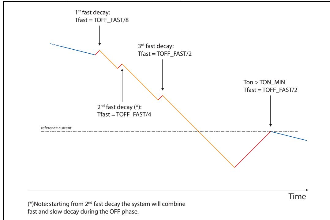
When two or more fast decays are performed with present target current, the control system adds a fast decay at the end of every OFF time, keeping the OFF state duration constant ( $t_{OFF}$  is split into  $t_{OFF,SLOW}$  and  $t_{OFF,FAST}$ ). When the current threshold is increased by a micro-step change (rising step), the system returns to normal decay mode (slow decay only) and the  $t_{FAST}$  value is halved.
