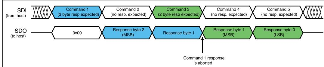
When a byte that does not correspond to a command is sent to the IC it is ignored and the **WRONG\_CMD** flag in the STATUS register is raised (see [Section 9.1.13](#)).
