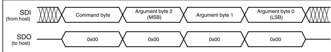
By default, the device returns an all zeroes response for any received byte, the only exceptions are GetParam and GetStatus commands. When one of these commands is received, the following response bytes represent the related register value (see [Figure 16](#)).
