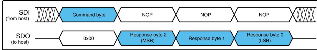
During response transmission, new commands can be sent. If a command requiring a response is sent before the previous response is completed, the response transmission is aborted and the new response is loaded into the output communication buffer (see [Figure 17](#)).
