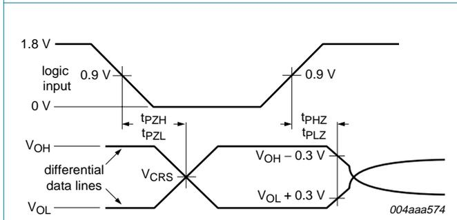
Fig 31. Timing of TX\_ENABLE to DP and DM
