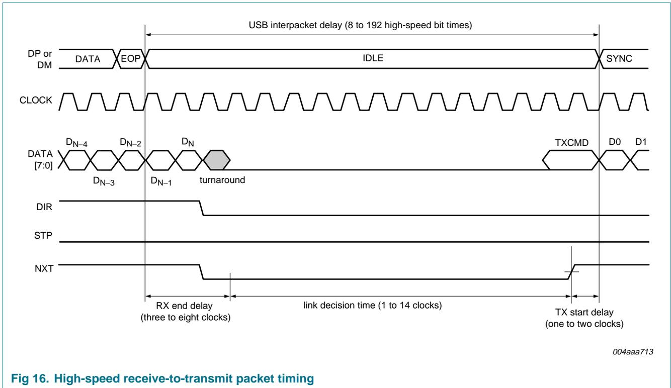
Fig 16. High-speed receive-to-transmit packet timing
