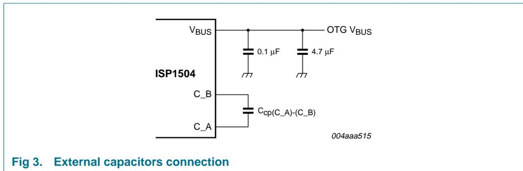
Fig 3. External capacitors connection
