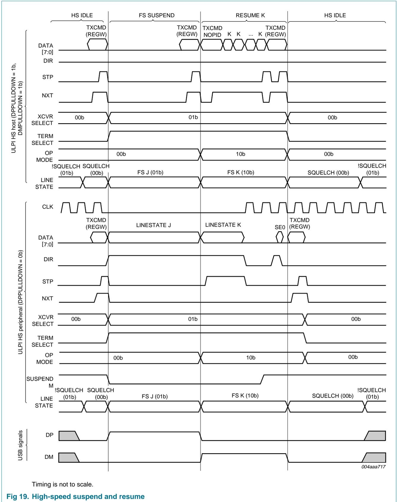
Fig 19. High-speed suspend and resume
