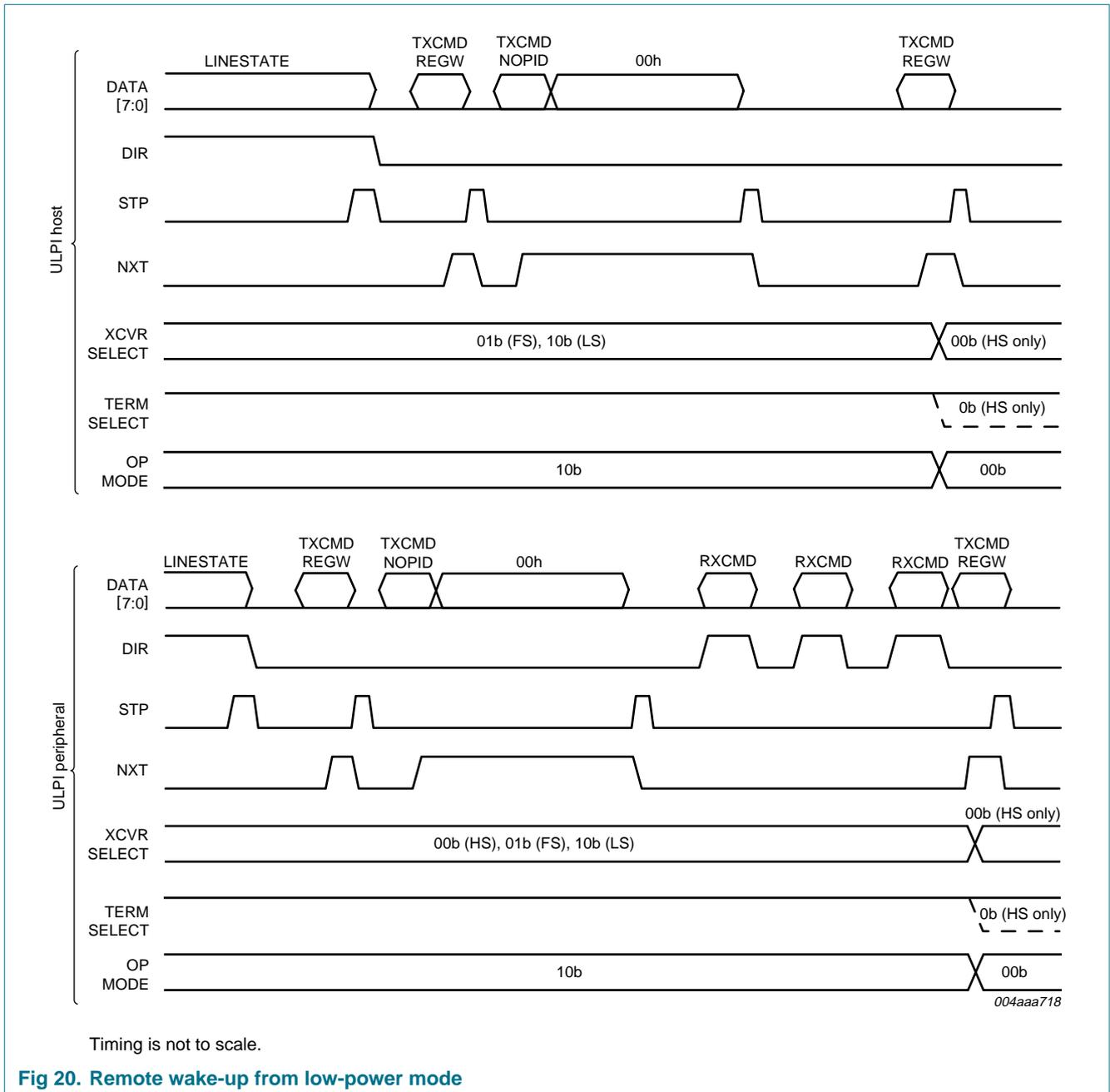
Fig 20. Remote wake-up from low-power mode
