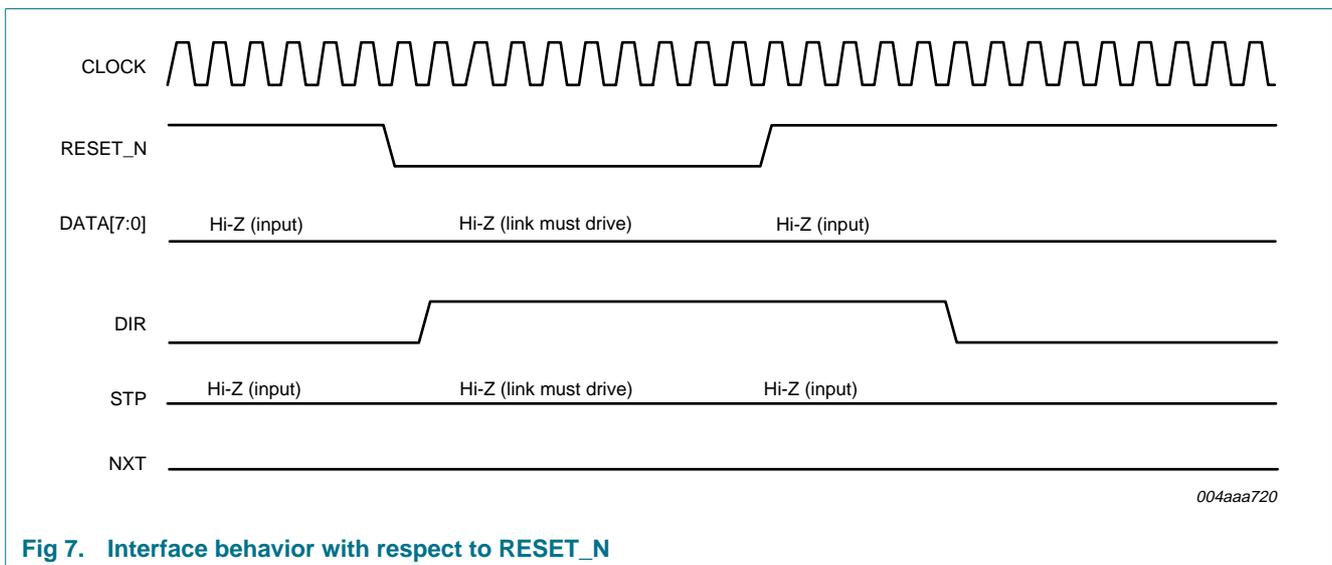
**Fig 7. Interface behavior with respect to RESET\_N**
