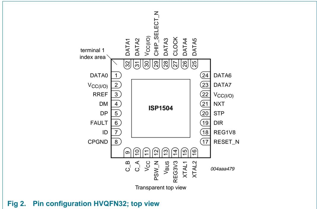
Fig 2. Pin configuration HVQFN32; top view
