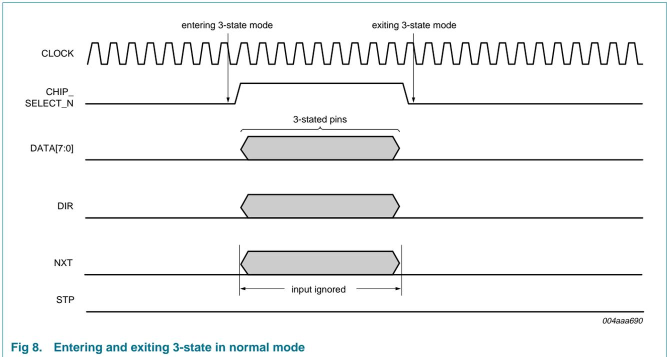
Fig 8. Entering and exiting 3-state in normal mode
