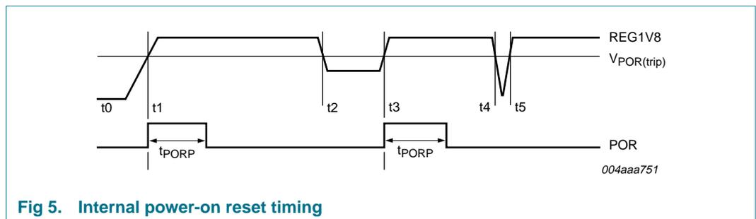
Fig 5. Internal power-on reset timing
