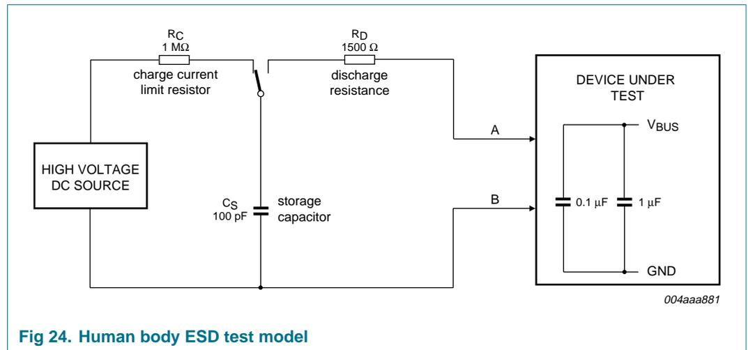
Fig 24. Human body ESD test model
