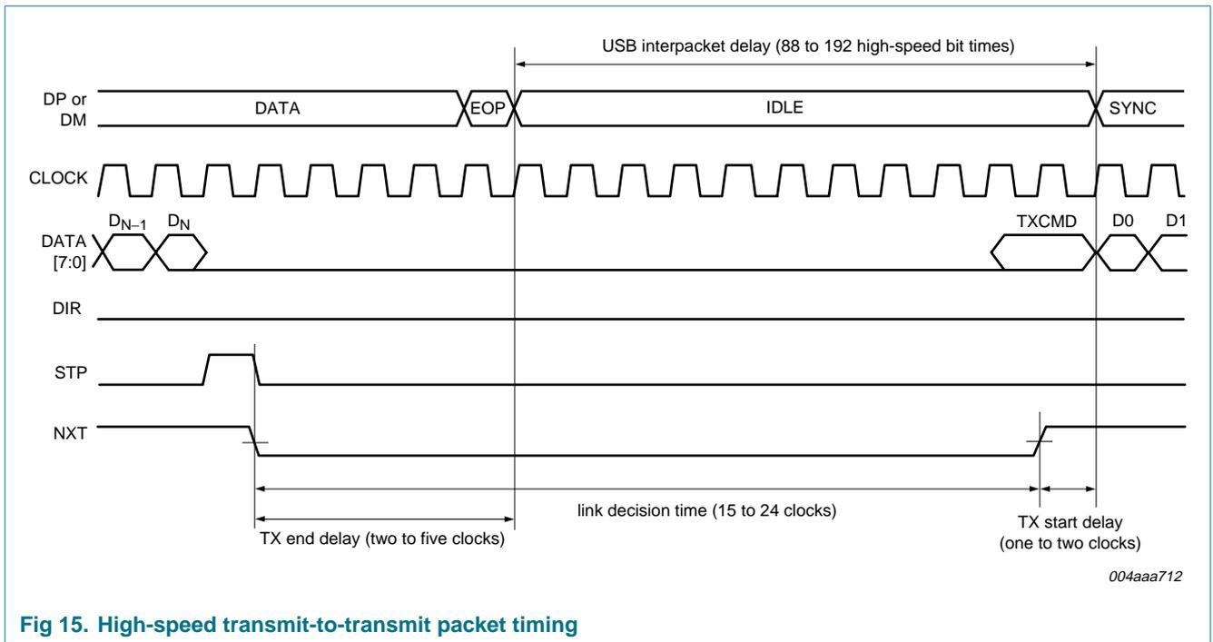
Fig 15. High-speed transmit-to-transmit packet timing
