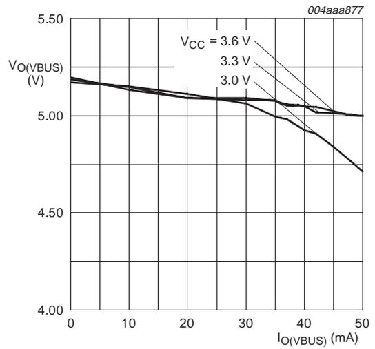
**Fig 26.  $V_{BUS}$  output voltage vs.  $V_{BUS}$  output current**
