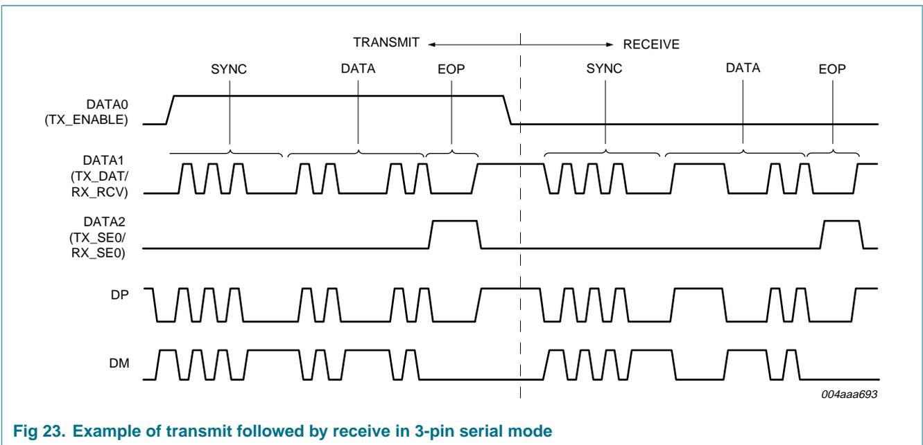
Fig 23. Example of transmit followed by receive in 3-pin serial mode
