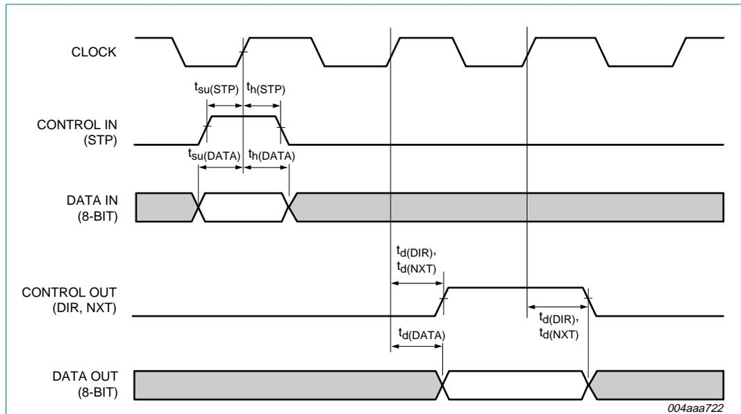
Fig 33. ULPI timing interface
