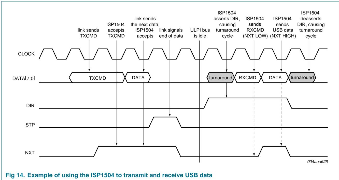
Fig 14. Example of using the ISP1504 to transmit and receive USB data
