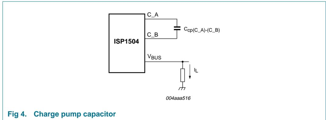
Fig 4. Charge pump capacitor
