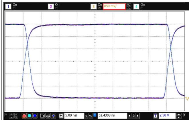
Figure 19. Eye Diagram at 25 Mbps, 5 V and 25°C
