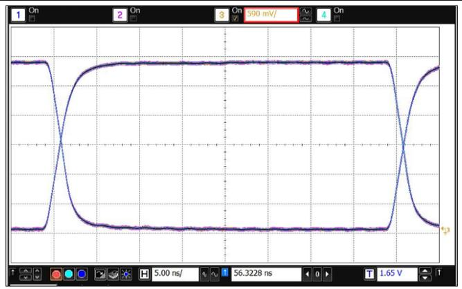
Figure 20. Eye Diagram at 25 Mbps, 3.3 V and 25°C
