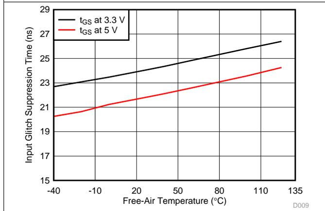
Figure 9. Input Glitch Suppression Time vs Free-Air Temperature
