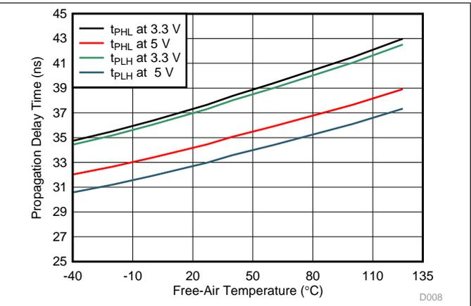
Figure 8. Propagation Delay Time vs Free-Air Temperature
