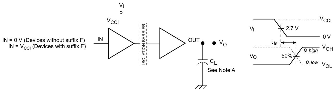
A.  $C_L = 15 \text{ pF}$  and includes instrumentation and fixture capacitance within  $\pm 20\%$ .
