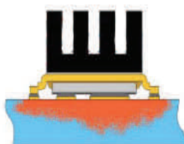
② Mounted to a PCB with small clip heatsink (still air)
