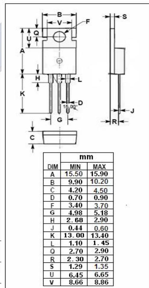
**isc N-Channel MOSFET Transistor**
