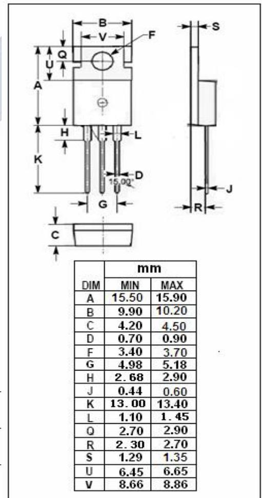
**isc N-Channel MOSFET Transistor**
