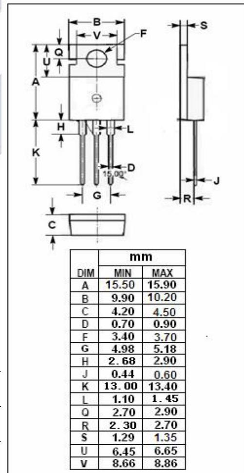
**isc N-Channel MOSFET Transistor****IPP060N06N, IIPP060N06N****ELECTRICAL CHARACTERISTICS** $T_c=25^\circ\text{C}$  unless otherwise specified
