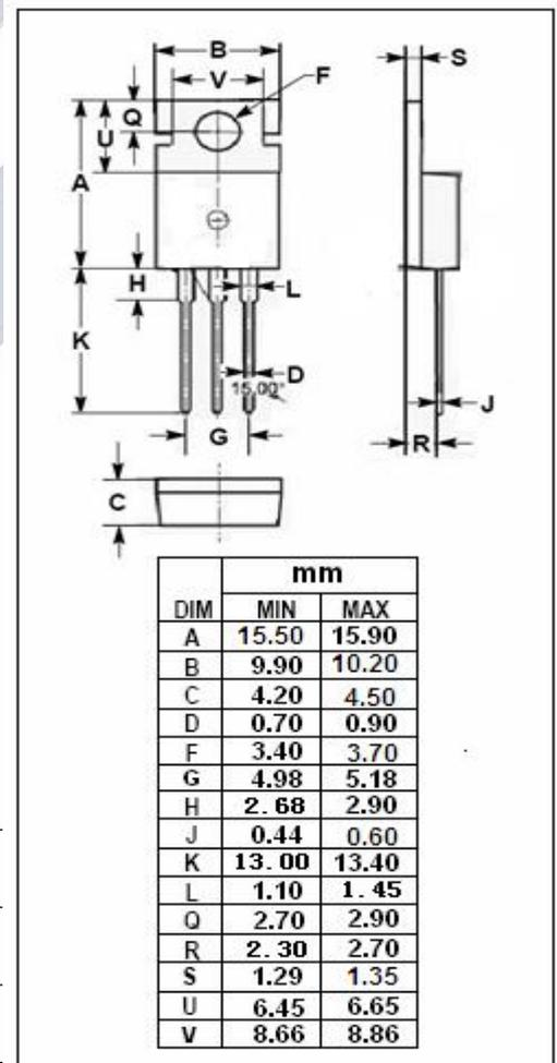
**isc N-Channel MOSFET Transistor      IPP037N06L3, IIPP037N06L3**
