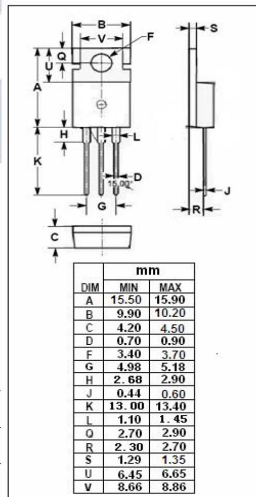
**isc N-Channel MOSFET Transistor IPP023NE7N3, IIPP023NE7N3****ELECTRICAL CHARACTERISTICS** $T_c=25^\circ\text{C}$  unless otherwise specified
