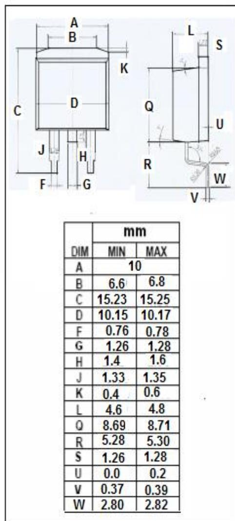
**isc N-Channel MOSFET Transistor****IPB60R165CP****ELECTRICAL CHARACTERISTICS** $T_c=25^\circ\text{C}$  unless otherwise specified
