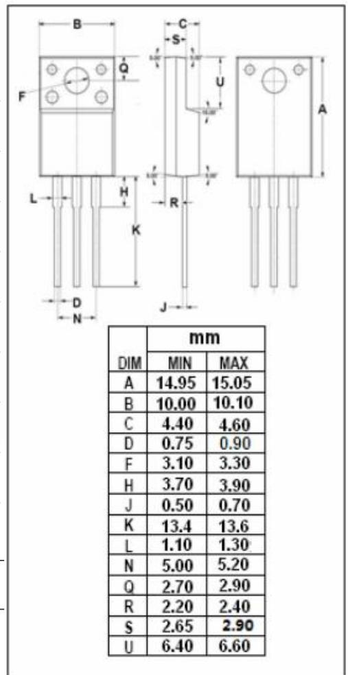
**isc N-Channel MOSFET Transistor**
