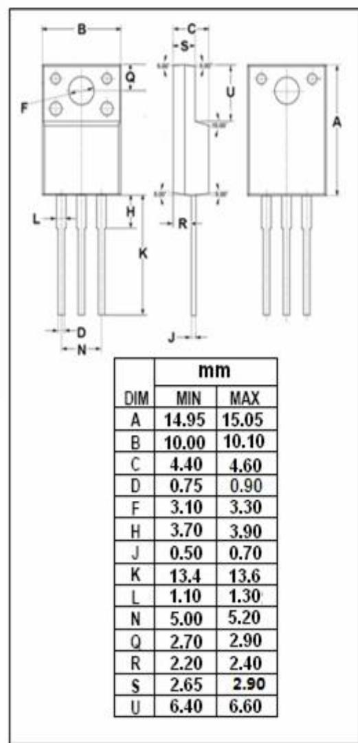
**Isc N-Channel MOSFET Transistor****IPA80R1K0CE****ELECTRICAL CHARACTERISTICS** $T_c=25^\circ\text{C}$  unless otherwise specified
